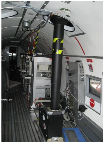
**Fig. 2.** The AMALi in a zenith-aiming airborne configuration on board the Polar 2 aircraft (left) and the Polar 5 aircraft (right).
