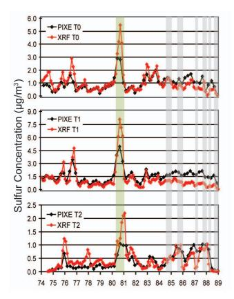
**Fig. 2.** Time series of the particulate Sulfur mass concentrations at the three sampling sites T0, T1, and T2 measured by PIXE and synchrotron XRF. Starting with T0, each site was located progressively farther from the Mexico City. During the day of transport 22 March, 2006 (DOY 80) large sulfur concentrations were observed at all three sites, indicating effective capture of the transport plume by particle samples. Additional transport days are indicated with the gray bars.
