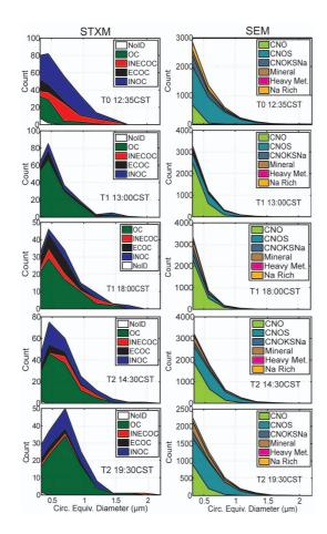
**Fig. 10.** Chemically resolved size distributions inferred from the STXM/NEXAFS (left) and CC-SEM/EDX (right) data sets for the samples collected at three sampling sites during 22 March, 2006. Bin widths are all equivalent.
