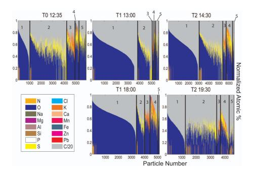
Fig. 9. Bar plot presentation of CCSEM/EDX data indicating composition of individual particles (each plot shows 5000-7000 particles) and relative particle-type contributions to the total sample characteristic for each of the samples collected at three sampling sites. Particle types are as follows: 1) CNO 2) CNOS 3) CNOSKNa 4) mineral dust 5) NaRich.
