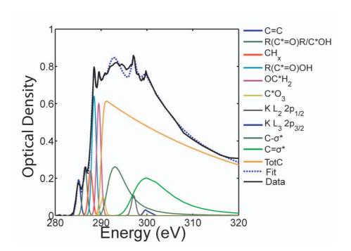
**Fig. 11.** Spectral deconvolution of the averaged C-edge spectrum of particles detected at the T0 site sample. The solid bold black line is the experimental data, the bold blue line is the best fit using the individual peaks labeled in the legend. A list of peak assignments and relative areas for all sites is given in Table 2.
