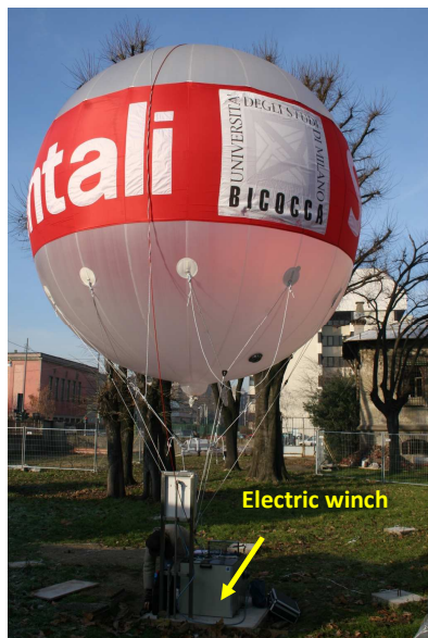
Fig. 1. The tethered balloon before launching at the sampling site and during a flight with its payload.
