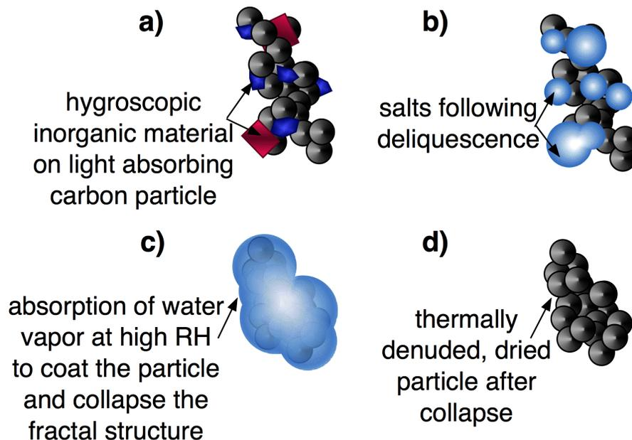
**Fig. 12.** Model of combustion product morphology for a carbonaceous particle with inorganic inclusions under increasing relative humidity conditions.
