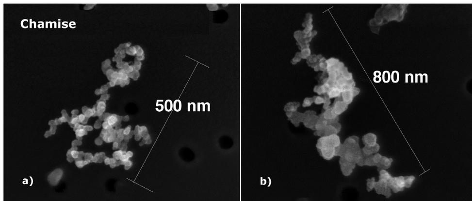
**Fig. 6.** Scanning electron microscope (SEM) images of **(a)** 500 nm and **(b)** 800 nm fractal-like soot chamise smoke particles sampled under ambient (dry) conditions without previous exposure to high RH. Individual monomers composing the fractal-like smoke particles are approximately 30 nm in diameter.
