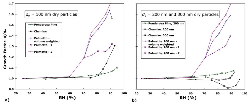
**Fig. 11.** Growth factor fraction:  $d/d_o$ . Hygroscopic growth of particle size (electrical mobility diameter) for **(a)** smaller and **(b)** larger smoke particles as a function of increasing relative humidity. Growth factor is the ratio of particle electrical mobility diameter,  $d$ , to dry diameter,  $d_o$ .
