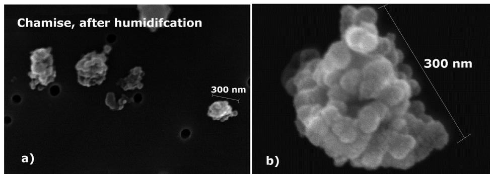
**Fig. 7.** Scanning electron microscope (SEM) images of collapsed (fractal dimension near 3) chamise smoke particles **(a)** sampled after humidification in excess of 80% RH. The diameter of each particle is approximately 300 nm. The close up image of a single humidified chamise smoke particle **(b)** has been magnified four times.
