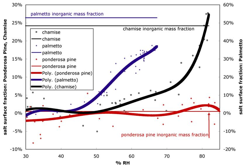
**Fig. 15.** Evaporation/condensation-implied surface coverage fraction. Surface coverage of liquid solution for each combustion product calculated using a model for photoacoustic absorption coefficient signals that includes evaporation-condensation and implied by measured values of  $\beta_{\text{abs}}$  under both ambient and high RH conditions.
