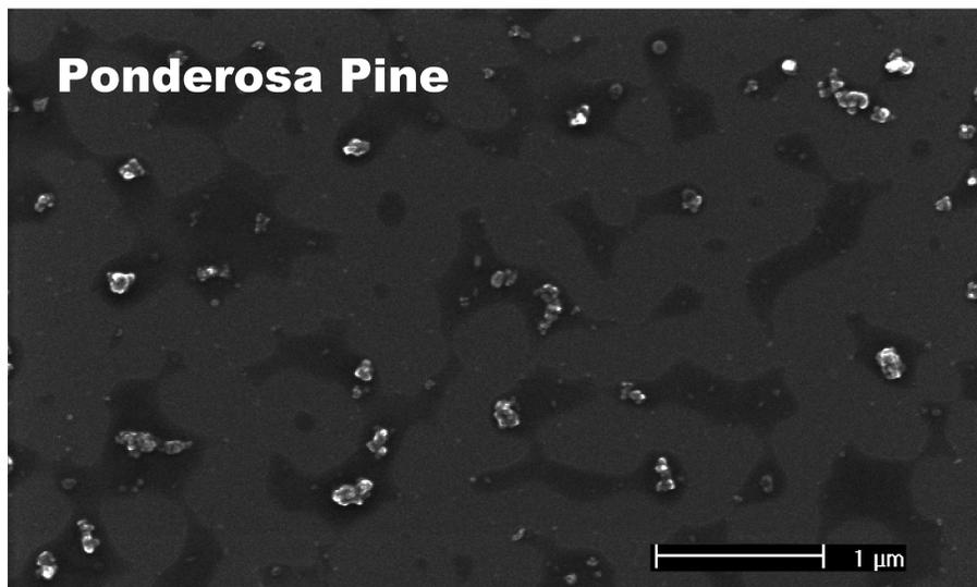
**Fig. 9.** SEM Image of ponderosa pine combustion particles. Particles are composed of organic materials with soot inclusions. Soot is always inside of liquid/oily organic substances. Almost no elements other than C and O are present, with the exception of occasional trace amounts of S and Cl.
