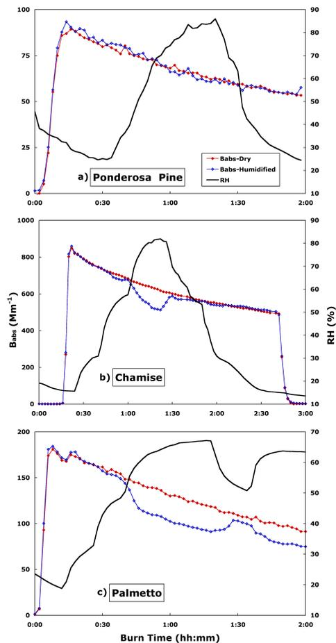
**Fig. 3.** Coefficients of absorption  $\beta_{\text{abs}}$  in  $\text{Mm}^{-1}$  measured by a photoacoustic instrument at 870 nm for a burn of (a) ponderosa pine, (b) chamise, and (c) palmetto fuel on two channels, including percent RH on the humidified channel.
