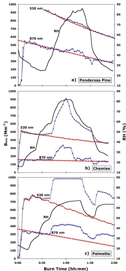
**Fig. 1.** Coefficients of scattering  $\beta_{\text{sca}}$  in  $\text{Mm}^{-1}$  measured by an integrating nephelometer (530 nm) and reciprocal nephelometer (870 nm) for a burn of (a) ponderosa pine, (b) chamise, and (c) palmetto fuel on two channels, including percent RH of the humidified channel. Measurements on the humidified channel are depicted in blue, while those on the ambient (dry) channel are in red.
