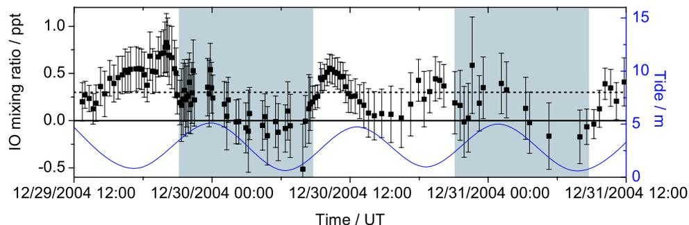
**Fig. 1.** Time series of IO measured by an active long-path DOAS setup along a 29 km absorption path in the marine boundary layer nearby Alcântara (2.4° S, 44.4° W), Brazil. The left abscissa shows inferred IO volume mixing ratio (boxes with error bars). The right abscissa correlates the local tides (blue line). The detection limit of the experiment is estimated  $\sim 0.3$  ppt (dotted black line). Nighttime is shaded grey.
