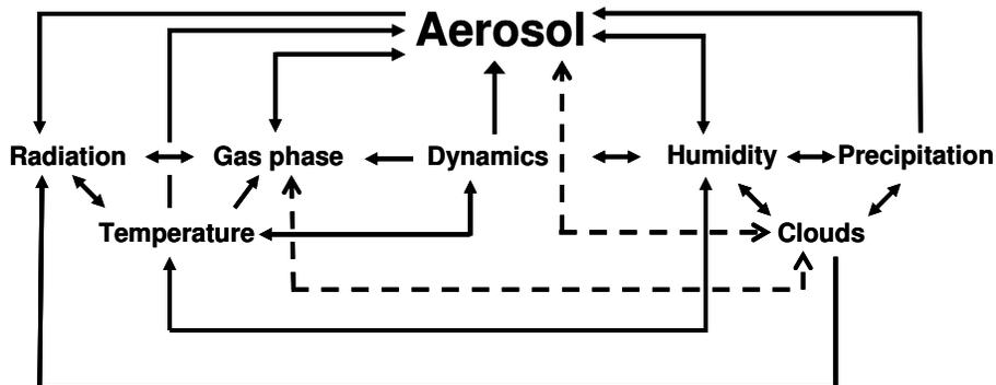
**Fig. 3.** Feedback processes that were taken into account. The dashed lines indicate interactions that are not taken into account.
