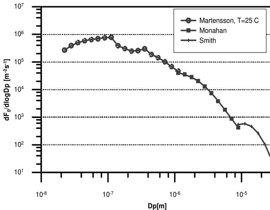
**Fig. 2.** The three parameterizations describing flux of particles per area of bubbles and second for chosen intervals for a sea surface temperature of 25°C and a wind speed of 9 m s<sup>-1</sup>.
