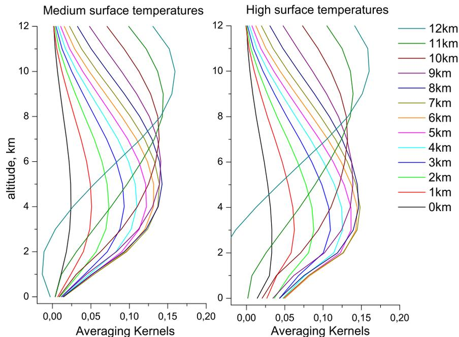
**Fig. 5.** IASI averaging kernels for European summer morning conditions. Averaging kernels for medium surface temperatures (between 15°C and 25°C) are shown in the left panel and for high surface temperatures (higher than 25°C) in the right panel.
