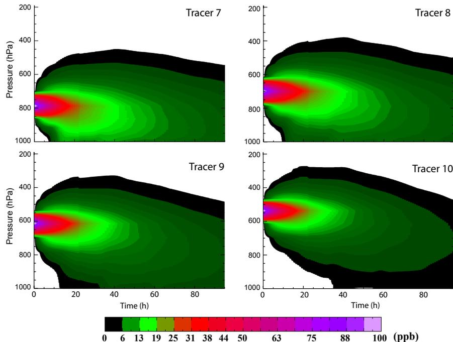
**Fig. 2a.** Time evolution (0–96 h) of vertical tracer distributions in summer 2003 for tracer 7 (870 hPa–800 hPa), tracer 8 (800 hPa–700 hPa), tracer 9 (700 hPa–620 hPa) and tracer 10 (620 hPa–650 hPa). For each tracer, concentrations (ppb) have been averaged over the whole geographical domain and over 21 4-day time periods.
