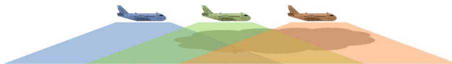
Fig. 3. Schematic of the geometry of the PSR along-track scans. The cartoon shows the swaths of three successive scan cycles, each labeled in different color. Each PSR swath spans \pm 70 degrees off the nadir. The aircraft translates approximately 5.85 km during a full PSR scan cycle. It can be seen from the cartoon that a scan cycle moderately overlaps with its succeeding scan, but hardly overlaps with its second succeeding scan.
