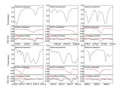
**Fig. 2.** Example of one spectrum observed by the ACE-FTS at 8 km in each microwindow selected for the retrieval of HCHO (top panels). The middle panel display the formaldehyde contribution to the atmospheric spectrum and the bottom panel display the residuals (observed-calculated) with the formaldehyde contribution included (red) or not (black) in the calculation.
