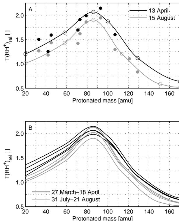
**Fig. 4.** Principle of the method for determining a relative transmission curve **(A)** and the relative transmission curves **(B)** derived from the calibrations shown in Fig. 3. The relative transmission coefficients (solid circles) were calculated using the measured sensitivities and the parameters used for fitting the curves (open circles) were determined according to the criteria explained in Sect. 2.4.3.
