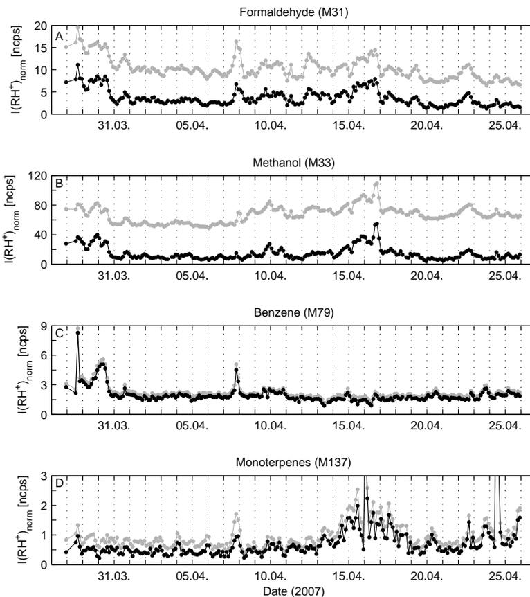
**Fig. 2.** Hourly averages of the normalized count rates of VOCs during the measurement period 27 March–26 April 2007. The black circles represent the normalized count rates that were calculated according to Eq. (6) and subsequently converted into volume mixing ratios (see Fig. 5). The grey circles show the normalized count rates when the VOC background signals were not subtracted.
