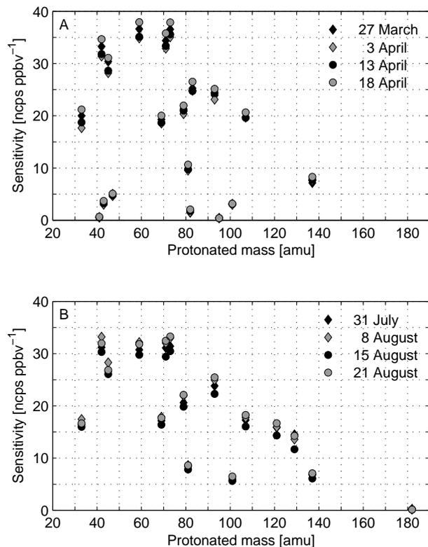
**Fig. 3.** Measured sensitivities for the VOCs in the calibration gas standards. The calibration setup and procedure were similar in all calibrations, except for the gas standard (Table 2). The calibrations were performed in 2007.
