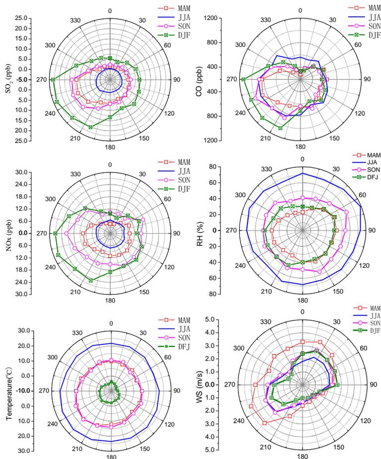
**Fig. 8.** Dependence of seasonal average SO<sub>2</sub>, NO<sub>x</sub>, CO, temperature, relative humidity (RH), and wind speed (WS) on wind direction.
