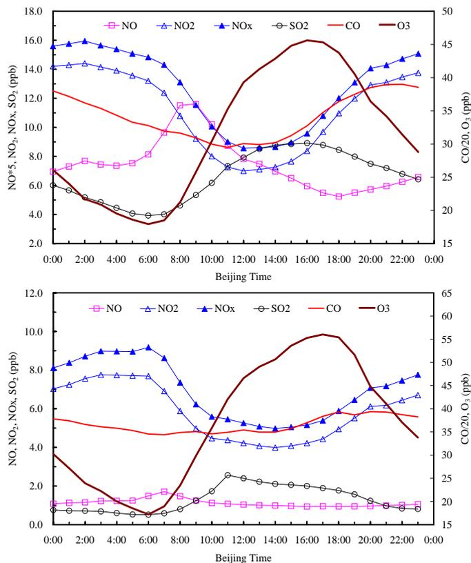
**Fig. 4.** Average diurnal variations of O<sub>3</sub>, NO/NO<sub>2</sub>/NO<sub>x</sub>, SO<sub>2</sub>, and CO at SDZ: the whole year (up), summer (bottom).
