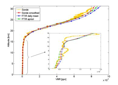
**Fig. 17.** Comparison of  $O_3$  vertical profiles at St-Denis on 16 September 2004 obtained from ground-based FTIR (blue diamonds) and  $O_3$  sonde (yellow dots). Green triangles indicate the a priori FTIR profile and red stars the sonde profile smoothed by the FTIR averaging kernels.
