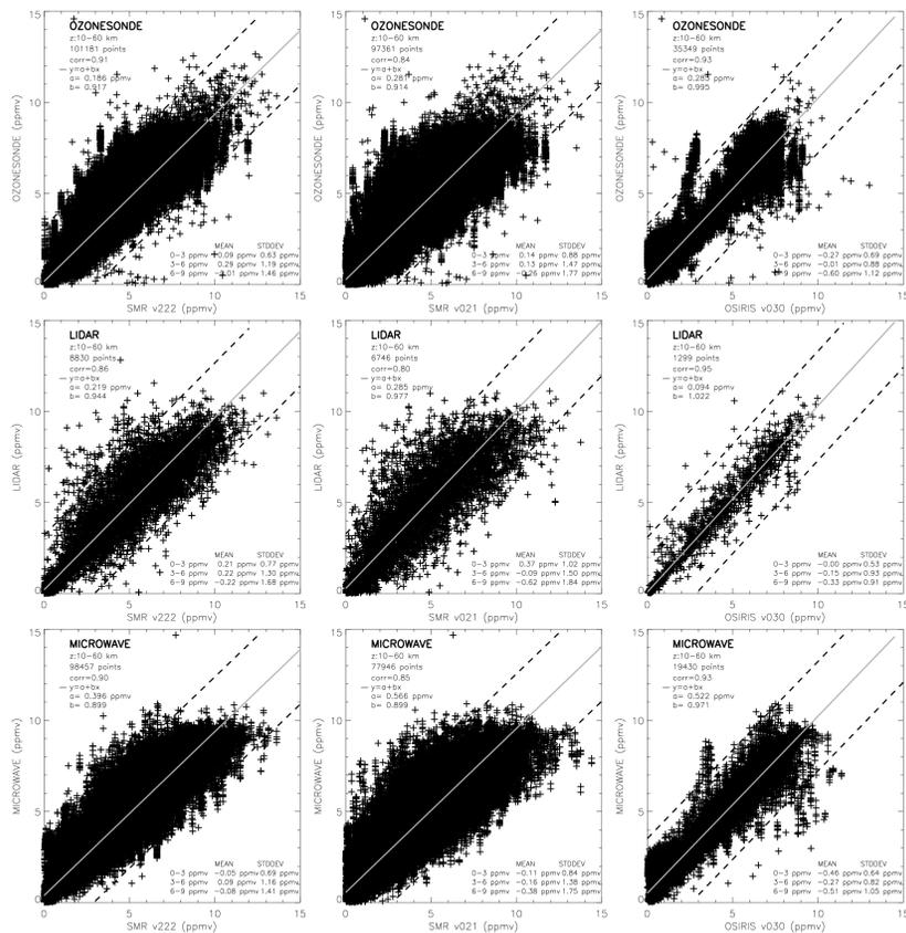
**Fig. 9.** Scatterplot of Odin/SMR and OSIRIS O<sub>3</sub> versus NDACC measurements. Left: Odin/SMR v222 data; middle: Odin/SMR v2.1 data; right: Odin/OSIRIS v3.0 data. Top: Ozonesonde, Middle: Lidar, Bottom: Micro-wave. Mean differences and standard deviations are indicated for the different ranges of the O<sub>3</sub> mixing ratio. The dotted lines delimit deviations of ±3 ppmv for clarity. The solid gray line indicates the linear fit to the data.
