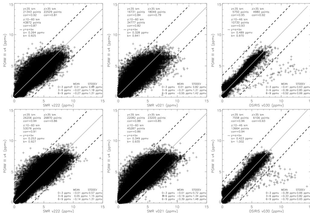
**Fig. 2.** Scatterplot of Odin/SMR and OSIRIS O<sub>3</sub> versus POAM III measurements. Left: Odin/SMR v222 data; middle: Odin/SMR v2.1 data; right: Odin/OSIRIS v3.0 data. Top: Southern hemisphere; bottom: Northern hemisphere. Mean differences and standard deviations are indicated for the different ranges of the O<sub>3</sub> mixing ratio. The dotted lines delimit deviations of ±3 ppmv for clarity. The solid gray line indicates the linear fit to the data.
