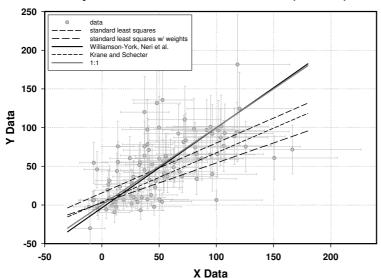
**Fig. 2.** Linear fits to data generated by sampling a Gaussian function with standard deviation of 10 units plus 30%, and adding the noise to the numbers 1 through 100. Fit parameters are shown in Table 3.
