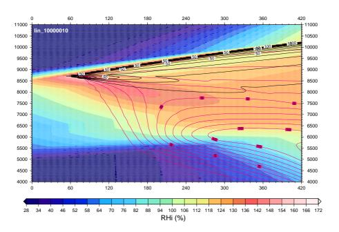
**Fig. 15.** Time evolution of the simulated cirrostratus lifted with a constant vertical velocity of  $w=0.05\,\mathrm{m\,s}^{-1}$ . The colours indicate relative humidity wrt ice, while lines indicate ice crystal number densities (black, in L<sup>-1</sup>) and ice water content (purple, in mg m<sup>-3</sup>).
