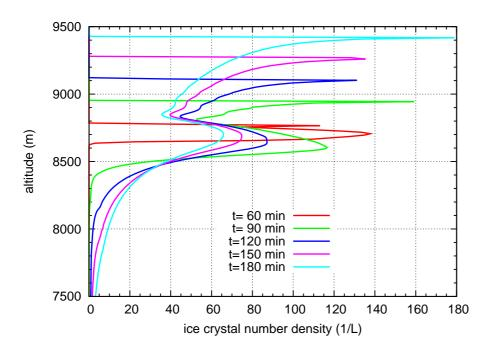
**Fig. 18.** Downward moving peak of ice crystal number density for the first nucleation event in the simulation with constant uplift of  $w=0.0\,\mathrm{m\,s}^{-1}$ . The peak is much more pronounced as in Fig. 17 due to higher ice crystal densities due to the stronger updraught.
