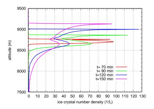
**Fig. 17.** Downward moving peak of high ice crystal number densities formed by the first homogeneous nucleation event at  $t \approx 60 \, \text{min}$  in the reference simulation (i.e. constant uplift of  $w = 0.05 \, \text{m s}^{-1}$ ). At the top of the cloud there is continuous nucleation, indicated by the high peak values of ice crystal number density.
