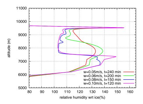
**Fig. 22.** Vertical RHi profile at the same altitude, i.e. at equivalent simulation times for all four simulations with different vertical updraught ( $w=0.05/0.06/0.08/0.1 \,\mathrm{m\,s}^{-1}$ ).
