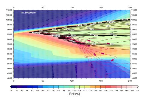
**Fig. 20.** Time evolution of the simulated cirrostratus lifted with a constant vertical velocity of  $w=0.08\,\mathrm{m\,s^{-1}}$ . The colours indicate relative humidity wrt ice, while lines indicate ice crystal number densities (black, in L<sup>-1</sup>) and ice water content (purple, in mg m<sup>-3</sup>).
