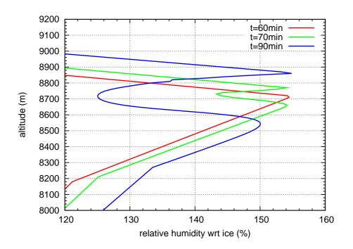
**Fig. 16.** Temporal evolution of the vertical RHi profiles for simulation time  $60 \le t \le 90$  min. The notch of the profile due to ice crystal growth is represented clearly, while the supersaturation at the cloud top remains.
