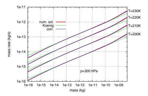
**Fig. 5.** Approximation of single ice crystal growth rates dm/dt (red) using the original Koenig ansatz (green) and the Koenig ansatz with our corrections (blue) for different temperatures  $(T=230/220/210/200 \, \text{K})$  and fixed pressure  $(p=300 \, \text{hPa})$ .
