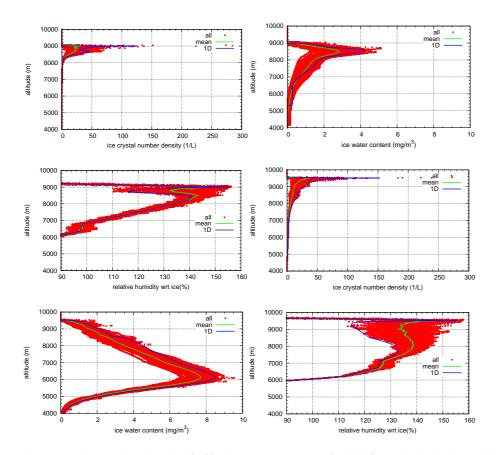
**Fig. 23.** Ice crystal number density (left), ice water content (middle) and relative humidity wrt ice (right) at  $t_s$ =120 min (top panel) and at  $t_s$ =240 min (bottom panel) for a constant updraught of w=0.05 m s<sup>-1</sup> and additional temperature fluctuations. The values at all grid points are indicated by the red dots, the mean value is represented by the green line and the blue line indicates the values of the corresponding 1-D simulation.
