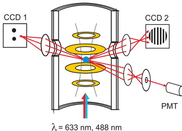
**Fig. 1.** Schematic of the electrodynamic balance. A three-wall glass chamber hosts four metal rings which supply the electric field needed for particle levitation. The particle is illuminated by two laser beams from below. The scattered light is collected in the near and far field view by two CCD cameras, and its intensity monitored by a photomultiplier (PMT).
