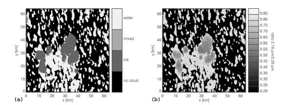
**Fig. 9.** Separation of thermodynamic phase. **(a)** cloud phase from the GCE data set for a  $60^{\circ}$  viewing zenith angle, GCE volume visible from that perspective only containing liquid water is labeled "water", volume containing only ice water content is "ice", volume containing both is "mixed". **(b)** Ratio of reflectance  $2.1/2.25\,\mu\text{m}$ . Due to differences in ice absorption, the cloud phase is separable.
