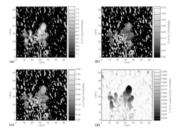
**Fig. 4.** Simulated cloud scanner observations: Based on GCE cloud data (compare Fig. 2) monochromatic reflectance for 0.87 (a), 2.1 (b), and  $2.25 \,\mu\text{m}$  (c), as well as emitted monochromatic radiance for  $10.8 \,\mu\text{m}$  (d). Solar zenith angle  $45^{\circ}$ , viewing zenith angle  $60^{\circ}$ . The lack of shadows is due to the fact that both sun and sensor have an azimuth of  $180^{\circ}$  ("south").
