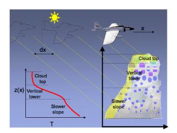
**Fig. 1.** Schematic depiction of the cloud scanner concept (taken from Martins et al., 2007): the sun is behind the sensor in the plane of observation. Reflected solar and near infra-red radiance is used to measure the particle size and phase of the outer layer of a convective cell. The measurement of thermal radiance provides height and additional geometrical information.
