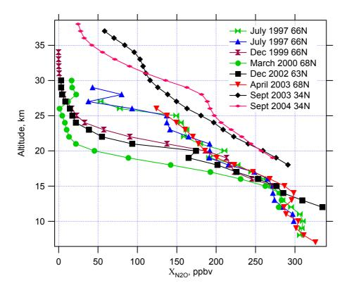
Fig. 3.  $N_2O$  measurements from the balloon-borne Mark IV Interferometer.
