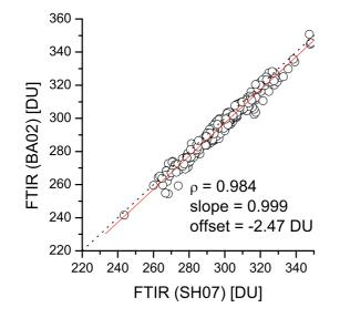
**Fig. 5.** Correlation between total column amounts for different FTIR approaches (a first similar to Barret et al. (2002) and a second according to Schneider and Hase (2007)). Black circles are individual measurements, red line linear regression lines of least squares fit.
