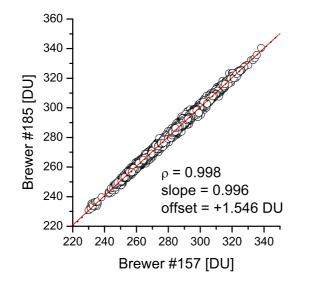
**Fig. 2.** Correlation between total column amounts of Brewer #157 and Brewer #185. Black circles are individual measurements, red line represents linear regression line of least squares fit.
