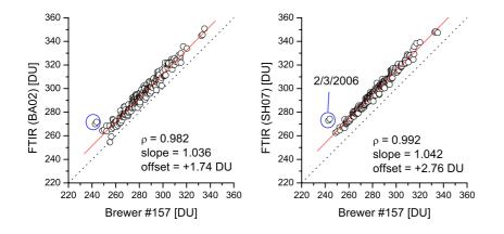
**Fig. 8.** Correlation between total column amounts of Brewer #157 and FTIR. Black circles are individual measurements, red lines linear regression lines of least squares fits. Left panel: correlation between Brewer and BA02 FTIR retrieval; right panel: correlation between Brewer and SH07 FTIR retrieval.
