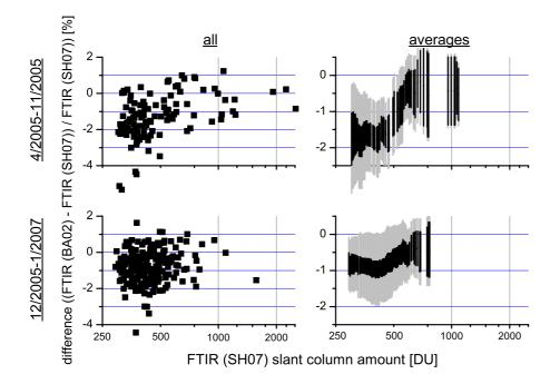
**Fig. 7.** Differences of total  $O_3$  measured by the different FTIR approaches (FTIR (BA02)–FTIR (SH07)) / FTIR (SH07)) versus slant column amounts. Content of panels, symbols, and colours is the same as in Fig. 4.
