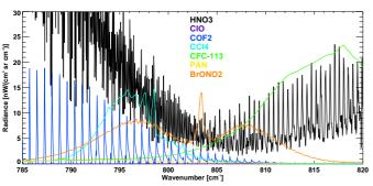
Fig. 1. Contributing trace gas signatures within the spectral range used for retrieval of BrONO2. The contributions are shown as radiances of each gas calculated independently of the other species. Calculations were made for a tangent altitude of 21 km using midlatitude night standard vmr-profiles (Remedios et al., 2007) and using the retrieved concentration of BrONO<sub>2</sub> from the 15° N-40° N night range (see Table 1 and Fig. 2).
