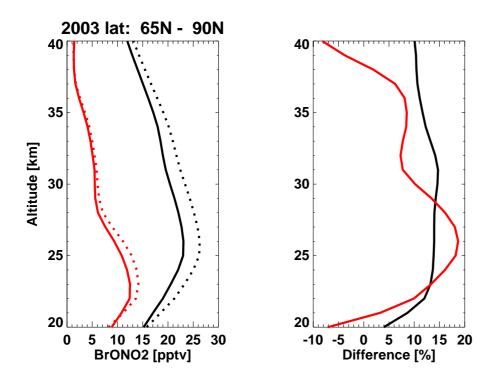
**Fig. 4.** Comparison of retrievals for latitude range 65–90° N in September 2003 using original BrONO<sub>2</sub> cross-sections by Orphal et al. (2008) (dotted) and results for temperature-adjusted cross-sections (solid) as described in Sect. 3.4.1. Daytime observations are in red while night-time measurements are in black.
