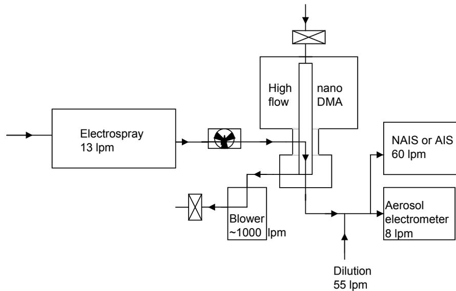
Fig. 1. (N)AIS mobility standard calibration set-up.
