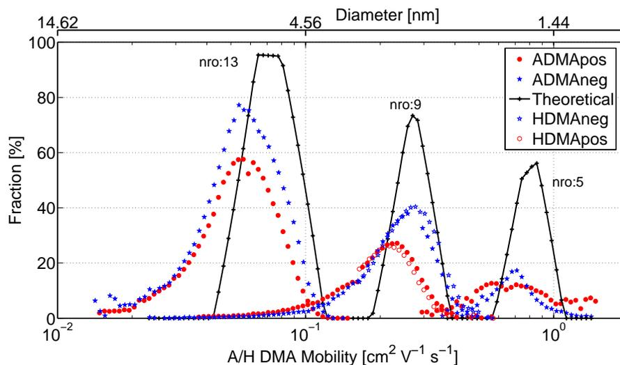
**Fig. 9.** Measured transfer functions for positive and negative ions and theoretical transfer functions for electrometers of the channels nro 5, 9, and 13. In theoretical transfer functions the ion losses in the inlet are additionally included, increasing the area compared to the measured transfer functions.
