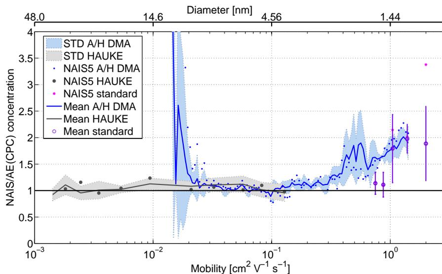
**Fig. 7.** Concentration of negative ions (average and standard deviation between (N)AISs, and NAIS5 measurement as an example) measured with (N)AIS as a function of Attoui/Herrmann and HAUKE DMA selected mobility using silver particles, charger ions, and molecular clusters (standards).
