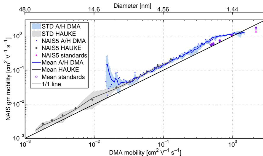
**Fig. 4.** Geometric mean mobility of positive ions (average and standard deviation between (N)AISs, and NAIS5 measurement as an example) measured with (N)AIS as a function of Attou/Herrmann and HAUKE DMA selected mobility of silver particles and charger ions, and monomobile mobility standards.
