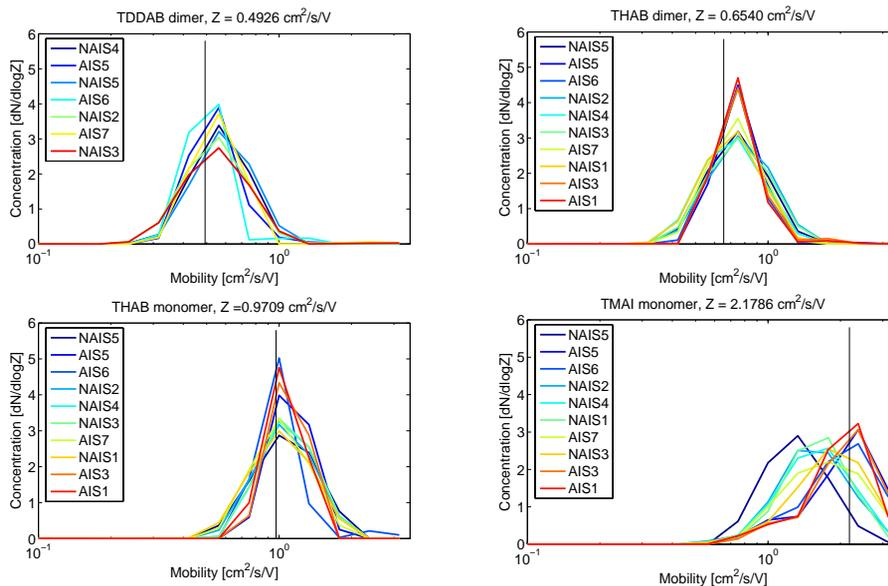
**Fig. 2.** Examples of four selected positive mobility standards measured with (N)AIS. The area of each measurement is normalised to unity and y-axis shows the normalised concentration and x-axis the mobility. The black vertical line shows the monomobile standard mobility.
