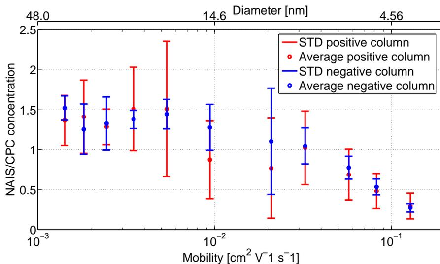
**Fig. 8.** Average concentration of all particles (charged+neutral) and standard deviation between the five NAISs as a function of HAUKE DMA selected mobility of silver particles. Particles measured in NAIS positive and negative column are presented separately.
