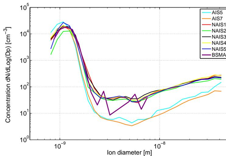
**Fig. 12.** Two day average negative ion number size distribution measured simultaneously with several (N)AISs.
