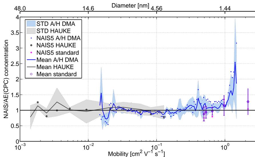
**Fig. 6.** Concentration of positive ions (average and standard deviation between (N)AISs, and NAIS5 measurement as an example) measured with (N)AIS as a function of Attoui/Herrmann and HAUKE DMA selected mobility of silver particles and charger ions, and monomobile mobility standards.
