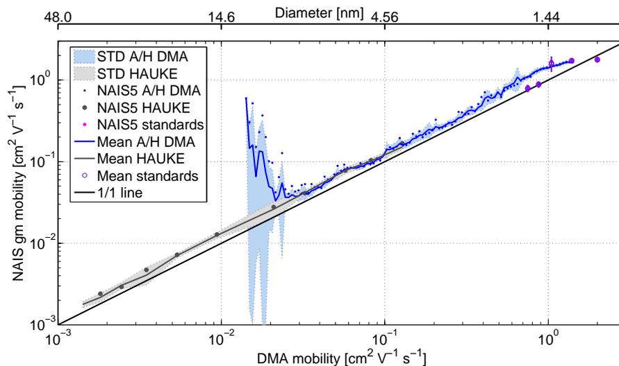
**Fig. 5.** Geometric mean mobility of negative ions (average and standard deviation between (N)AISs, and NAIS5 measurement as an example) measured with (N)AIS as a function of At-toui/Herrmann and HAUKE DMA selected mobility of silver particles, charger ions, and molecular clusters (standards).
