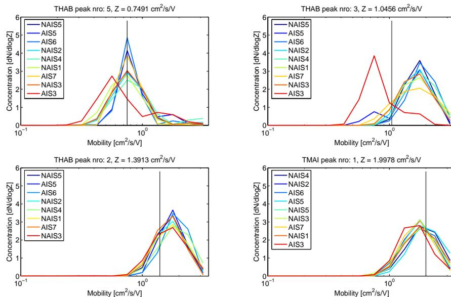
**Fig. 3.** Examples of four selected negative mobilities (unidentified standard peaks) measured with (N)AIS. The area of each measurement is normalised to unity and y-axis shows the normalised concentration and x-axis the mobility. The black vertical line shows the monomobile standard mobility.
