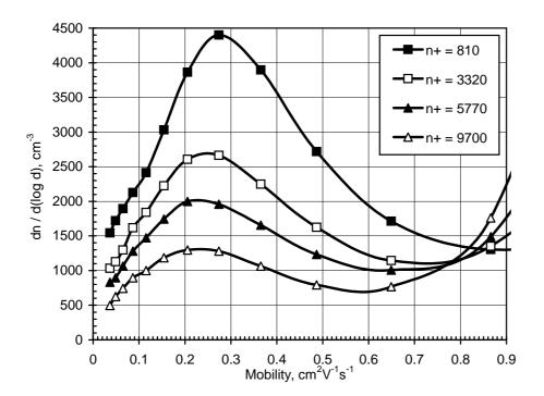
**Fig. 2.** Effect of particle neutralization on the mobility distribution of the negative balloelectric ions  $(0.03-0.5\,\mathrm{cm^2\,V^{-1}\,s^{-1}})$ . The curves correspond to the indicated on the legend concentrations  $(\mathrm{cm^{-3}})$  of positive cluster ions of the mobility above  $0.56\,\mathrm{cm^2\,V^{-1}\,s^{-1}}$ . The concentration  $n^+$ =810 cm<sup>-3</sup> is the natural level of ionization in the experiment room.
