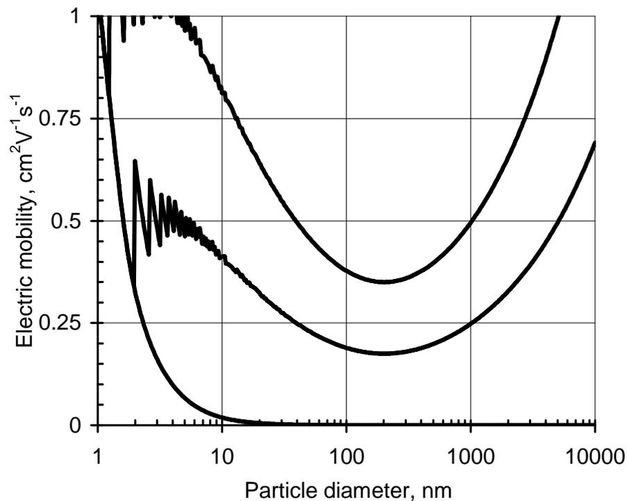
**Fig. 1.** Electric mobility of charged water droplets at the temperature of 10°C and the pressure of 1000 mb according to Tammet (1995). Curves from the top to bottom correspond to the droplet charge  $q_R$  (the Rayleigh limit),  $q_R/2$ , and the single elementary charge.
