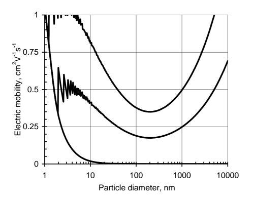
**Fig. 1.** Electric mobility of charged water droplets at the temperature of 10 $^{\circ}$ C and the pressure of 1000 mb according to Tammet (1995). Curves from the top to bottom correspond to the droplet charge  $q_R$  (the Rayleigh limit),  $q_R/2$ , and the single elementary charge.
