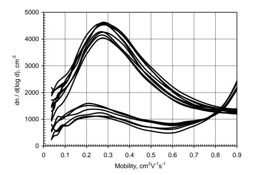
**Fig. 3.** Individual ten-minute negative ion mobility distributions, used in calculating the averages for Fig. 2. Upper 9 curves are measured at  $n^+$ =810 cm<sup>-3</sup> and lover 6 curves at  $n^+$ =9700 cm<sup>-3</sup>.
