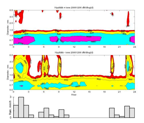
Fig. 4. Intermediate ion size distributions and rain intensity in Hyytiälä, 6 December 2006. Air temperature varied between 5.0 and 8.5°C and relative humidity varied between 83 and 96% during the day.
