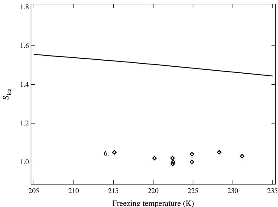
**Fig. 7.** Ice saturation ratio  $S_{ice}$  as a function of freezing temperature for heterogeneous ice nucleation onto solid ammonium sulfate particles in this study (open diamonds). The thick solid line represents the homogeneous ice nucleation model developed by Koop et al. (2000) and the thin solid line is an  $S_{ice}$  of 1. The IR spectra shown in Figure 6 were used to produce the point highlighted with the “6”.
