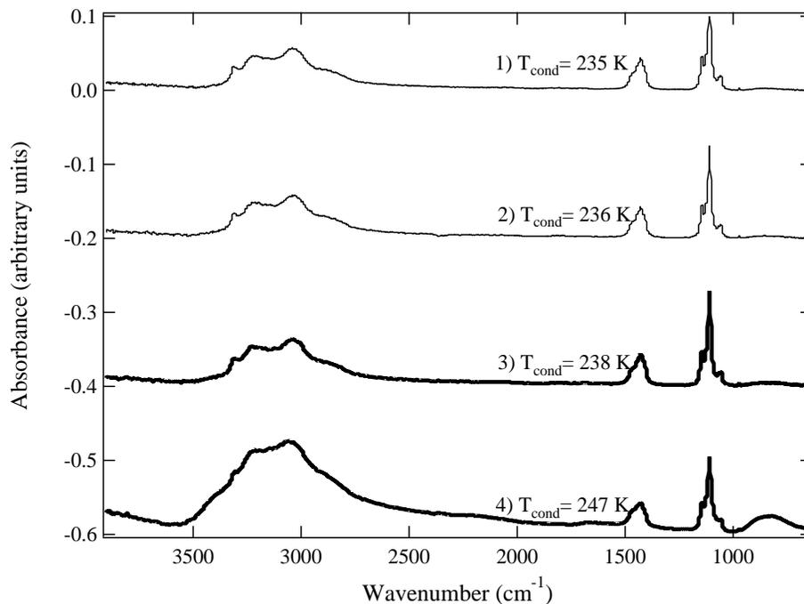
**Fig. 6.** IR spectra of effloresced ammonium sulfate particles (preconditioned using two 98 wt% sulfuric acid baths) as the temperature was raised in the conditioning region from 235 K to 247 K. The observation region was held at a constant 215 K. The onset of ice nucleation occurred when the conditioning region temperature reached 238 K. The spectra in which ice is present are highlighted with thicker lines and all spectra are offset for clarity.
