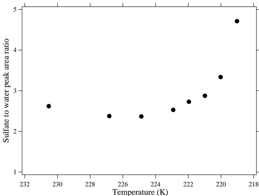
**Fig. 3.** Sulfate to water peak area ratio versus temperature for the homogeneous ice nucleation experiment described in Fig. 2. At 219 K, a significant increase in the peak area ratio occurred which signaled the onset of ice formation.
