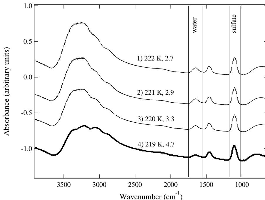
**Fig. 2.** IR spectra of aqueous ammonium sulfate particles (preconditioned using a distilled water bath) as the temperature was dropped in the observation region from 222 K to 219 K. The onset of ice nucleation occurred at 219 K and caused a substantial increase in the sulfate to water peak area ratio (4.7, peaks highlighted with vertical lines). The spectrum in which ice is present is denoted with a thicker line and all spectra are offset for clarity.
