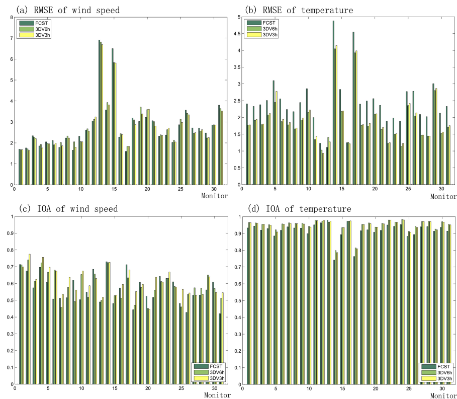
Fig. 7. The RMSE and index of agreement (IOA) calculated in FCST, 3DV6h, and 3DV3h against the measurements in terms of surface wind speed and temperature at the surface monitoring sites during 13–16 April 2003.
