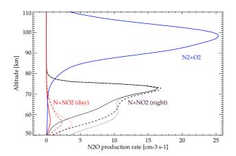
**Fig. 10.** Estimated EEP-related  $N_2O$  productions by Reaction (R1) at polar night (solid black line) and day (SZA=80°) conditions (solid red line), as well as by Reaction (R2) (solid blue line) for the nominal scenario. Dashed and dotted lines represent  $N_2O$  productions for the "high  $NO_x$ " scenario combined with the nominal and the "strong descent" temperature scenarios, respectively (only Reaction R1). See text for further details.
