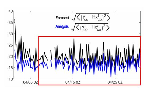
**Fig. 15.** Six-hourly root-mean-square error (in ppbv) of DART/CAM CO forecast (black) and analysis (blue) relative to MOPTT retrievals averaged over the INTEX-B domain.
