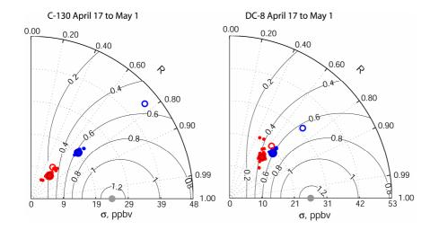
**Fig. 9a.** DART/CAM model skills relative to INTEX-B flight observations (gray). The blue dots represent the model skills for each ensemble member of DART/CAM with MOPITT assimilation (COASSIM) while red dots correspond to DART/CAM without MOPITT assimilation (REFSIM). Large filled circles correspond to ensemble-mean of analyses with the unfilled circles representing the total RMSE (see Fig. 9b).
