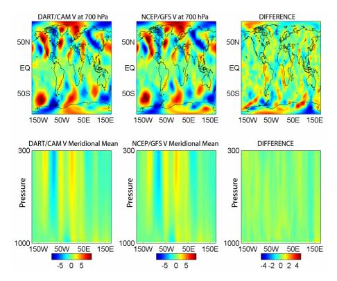
**Fig. 8b.** Global comparison of April 2006 mean horizontal wind component (V) in m/s from DART/CAM assimilation and NCEP/GFS forecast/analysis product (regridded to 2°×2.5°). The upper panels correspond to 700 hPa distribution while the lower panels correspond to merid-ional distribution (vertical axis in hPa).
