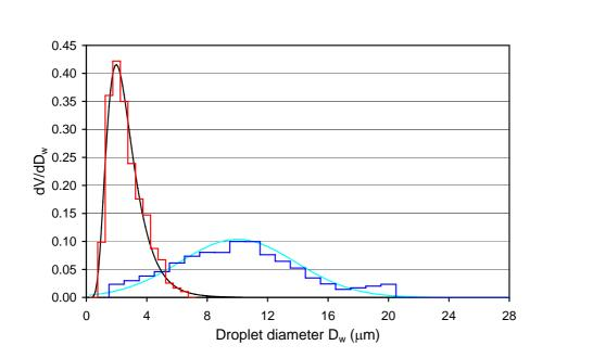
**Fig. 1.** Normalized volume distribution of water-in-oil emulsions: microscopically determined distributions are given in red (small droplets) and dark blue (large droplets), fitted functions in black (lognormal distribution, small droplets) and light blue (normal distribution, large droplets).
