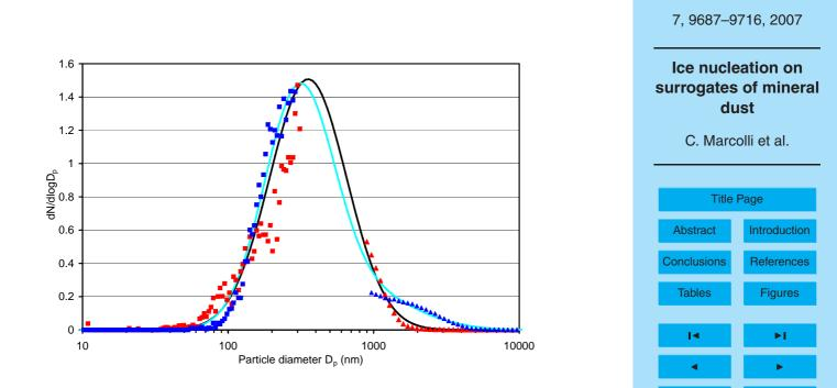
**Fig. 2.** Normalized number distributions of Arizona test dust (ATD): measured size distributions are given in red (fine ATD; squares: scanning mobility particle sizer (SMPS), triangles: aero-dynamic particle spectrometer (APS)) and dark blue (coarse ATD; squares: SMPS, triangles: APS). Fitted distributions are in black (fine ATD) and light blue (coarse ATD).
