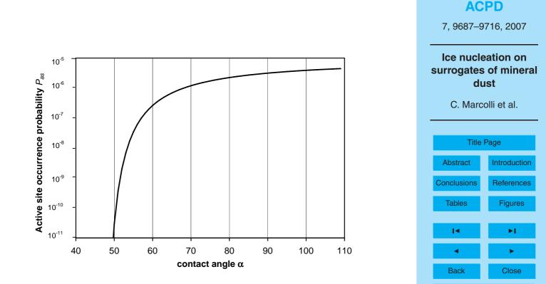
**Fig. 6.** Occurrence probability of active sites as a function of contact angle  $\alpha$ . This function was used to calculate the freezing curves in Figs. 4d and 5d.
