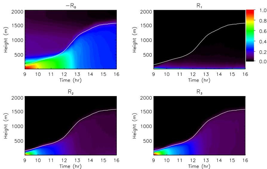
**Fig. 10.** Time-height plots of the radioactive decay  $-R_0$ ,  $R_1$ ,  $R_2$  and  $R_3$ . The contributions have been made dimensionless using their maximum values. The daytime boundary layer depth, defined as the altitude where the sensible heat flux is minimum, is also shown using solid white lines.
