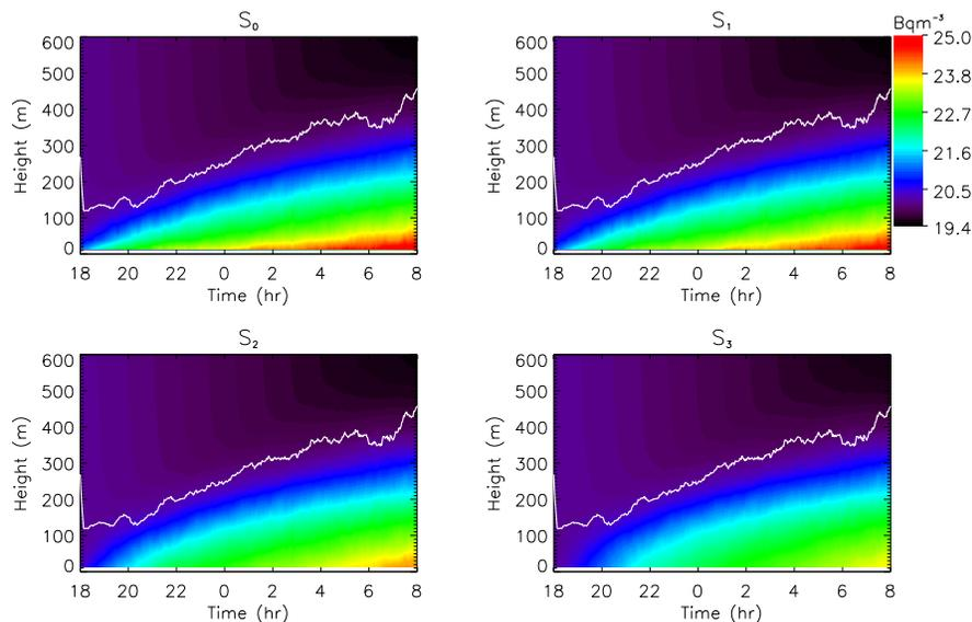
**Fig. 5.** Time-height plots of the radon and its short-lived daughter concentrations. The boundary layer depth is shown using a solid line. It is defined as the height where the turbulent heat flux is 5% of its surface value (Estournel and Guedalia, 1985).
