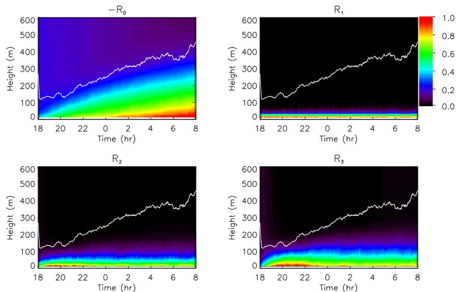
**Fig. 7.** Time-height plots of the radioactive decay contributions  $R_i$ . The contributions have been made dimensionless using their maximum values. The boundary layer depth is shown using a solid line. It is defined as the height where the turbulent heat flux is 5% of its surface value (Estournel and Guedalia, 1985).
