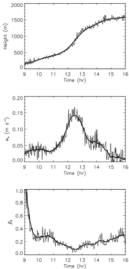
**Fig. 11.** Boundary layer depth  $z_i$ , entrainment velocity  $w_e$  and  $\beta_\theta$  time evolutions. Smoothed results are also shown in thick solid lines.
