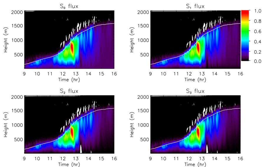
**Fig. 9.** Time-height plots of the radon and its short-lived daughter dimensionless fluxes. The fluxes have been made dimensionless using their maximum values. The daytime boundary layer depth, defined as the altitude where the sensible heat flux is minimum, is also shown using a solid line.
