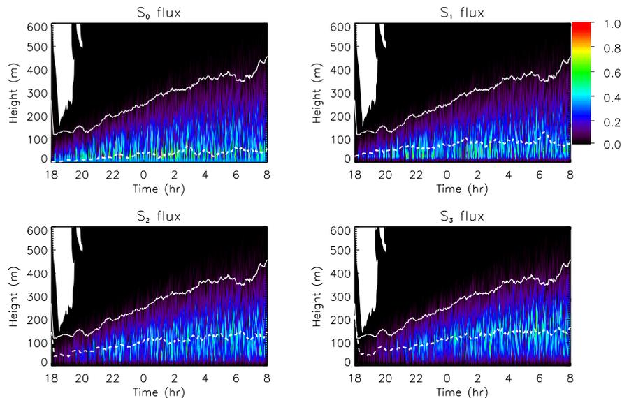
**Fig. 6.** Time-heightplots of the radon and its short-lived daughter dimensionless fluxes. The fluxes have been made dimensionless using their maximum values. The boundary layer depth is shown using a solid line. It is defined as the height where the turbulent heat flux is 5% of its surface value (Estournel and Guedalia, 1985). The areas in white represents downward fluxes. The localisation of the maximum fluxes is shown in dashed lines.
