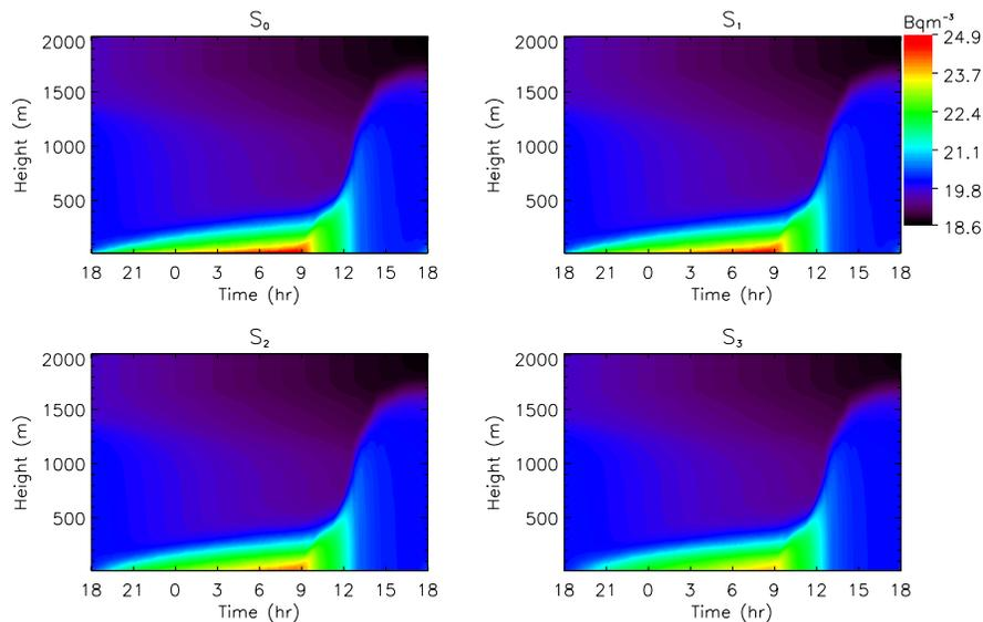
**Fig. 3.** Time-height plot of  $S_0$  and its progeny.
