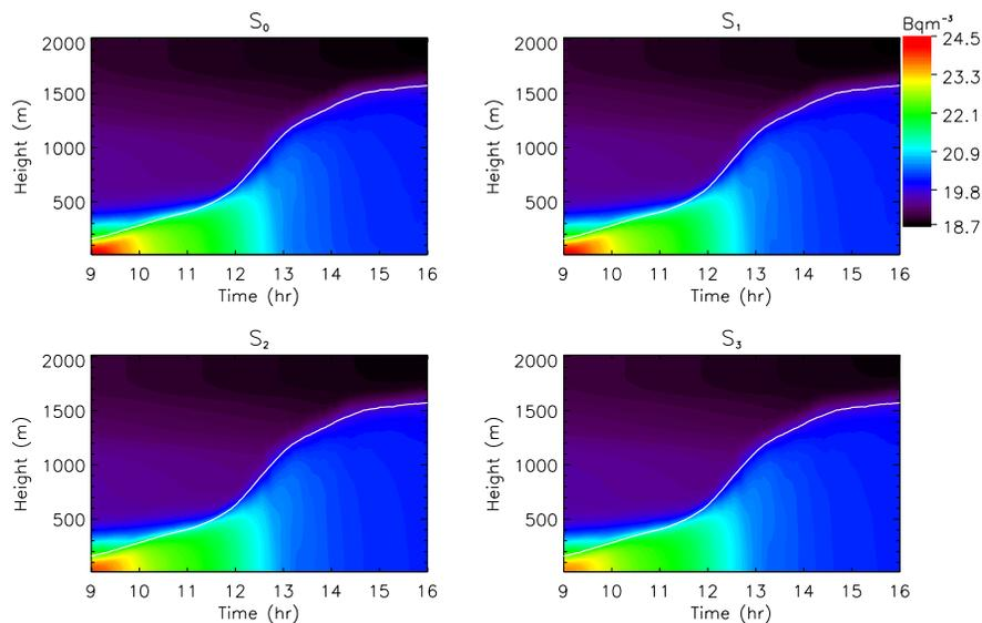
**Fig. 8.** Time-height plots of the radon and its short-lived daughter concentrations. The daytime boundary layer depth, defined as the altitude where the sensible heat flux is minimum, is also shown using solid white lines.
