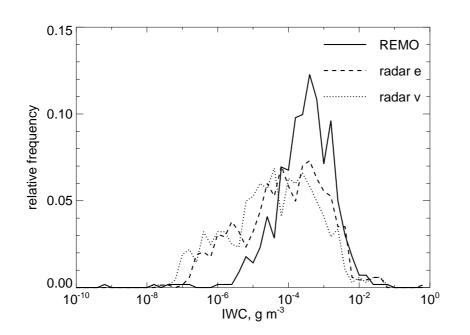
**Fig. 24.** Probability density functions of IWC derived from REMO and from cloud radar (using the algorithm of Hogan et al., 2006) in the range of 6000 m to 10 000 m. The abbreviations "e" and "v" stand for the Z-IWC – algorithms optimizing the expected value and the variance of IWC, respectively.
