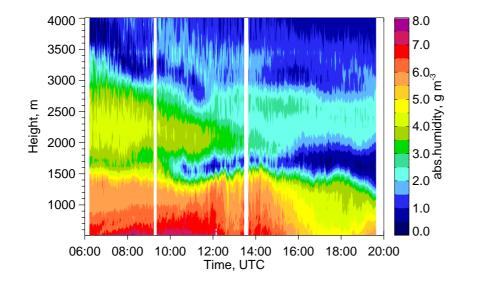
Fig. 2. Time-height cross-section of absolute humidity on 29 May 2003. The values are averages over 3 min.
