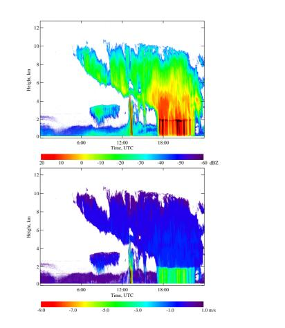
**Fig. 5.** Time-height cross-sections of the effective radar reflectivity factor (upper panel) and the Doppler velocity (lower panel) on 4 June 2004.
