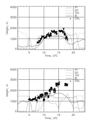
**Fig. 17.** ABL height derived from REMO and from DIAL on 10 June 2003 (top) and 7 June 2004 (bottom). The model ABL height is derived from the gradient of potential temperature (PT), of specific humidity (QD), of turbulent kinetic energy (TKE) and from static stability (BL, see chapter 2).
