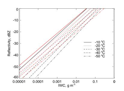
**Fig. 9.** Derivation of ice water content from cloud radar reflectivity by relations of IWC and dBZ according to Hogan et al. (2006), stratified by temperature, black lines: "best expected value", red lines: "best variance".
