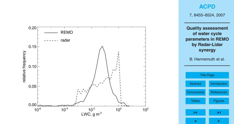
**Fig. 23.** Frequency distributions of LWC derived from REMO and from cloud radar (using the algorithm of Krasnov and Russchenberg, 2003) in the height range of 1800 m to 3000 m.
