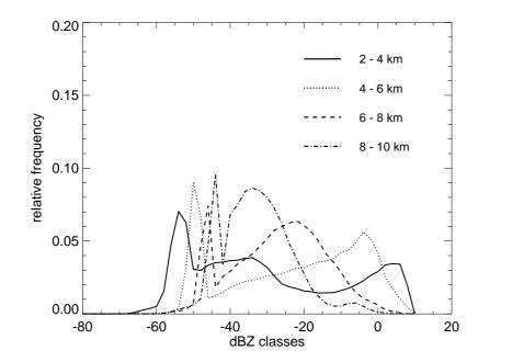
Fig. 1. Frequency distribution of radar reflectivity at different heights.
