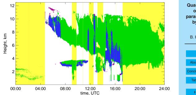
**Fig. 7.** Cloud mask derived from radar and lidar on 4 June 2004. Meaning of colors: yellow: no lidar observation, green: radar cloud, blue: radar and lidar cloud, purple: lidar cloud.
