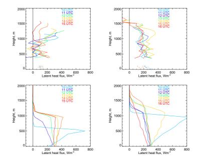
**Fig. 19.** Vertical profiles of latent heat flux on 30 May 2003 (left), and 9 June 2003 (right). Top: lidar measurements, bottom: REMO simulations.
