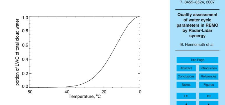
**Fig. 10.** Partioning of predicted total cloud water into liquid cloud water and ice cloud water in REMO5.5.
