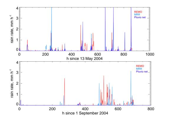
Fig. 25. Time series of rain rates for two measuring campaigns from REMO (red), MRR (light blue), and rain gauge network (blue).
