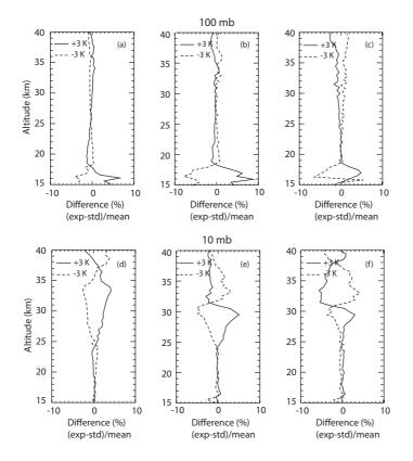
**Fig. 8.** Panels **(a)**, **(b)**, and **(c)** show the result of perturbing the input temperature value at 100 mb by 3 K (solid lines) and -3 K (dashed). Percent differences for the 1020-nm extinction (a), 525-nm extinction (b) and 525-nm/1020-nm ratio (c) are (experimental - standard)/mean with the meanings as in Fig. 6. Same suite of measurements and cloud clearing is also the same as in Fig. 6. Panels **(d)**, **(e)**, and **(f)**: same at the 10 mb level.
