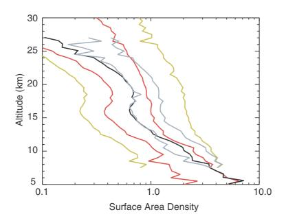
**Fig. 15.** This figure shows the comparison of operational SAGE II SAD (black) with the Method 1 SAD using 525-nm aerosol extinction coefficient (red) and the Method 2 SAD using the 525 and 1020 nm channels (gold) and the Method 2 SAD computed using the channels at 525 and 1020 nm plus a pseudo-infrared channel (grey).
