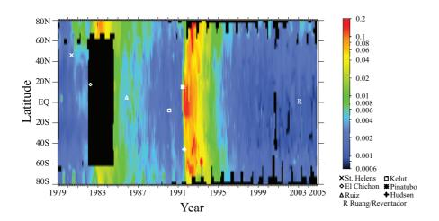
**Fig. 1.** The 1020-nm stratospheric optical depth from SAM II, SAGE, SAGE II and SAGE III for the period from January 1979 through the end of 2004. Between the June 1991 Pinatubo eruption and mid 1993, aerosol extinction coefficient profiles are supplemented by lidar data following the method described in Thomason and Peter (2006).
