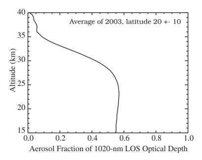
**Fig. 5.** Fraction of the measured slant path optical depth in the 1020-nm channel that is attributed to aerosol. All events between  $10^{\circ}$  N and  $30^{\circ}$  N in 2003 are included in the average shown here. Under the conditions of interest the  $H_2SO_4$ - $H_2O$  aerosol is expected to fully evaporate at temperatures above ~238 K, corresponding to altitudes between 35 km and 40 km.
