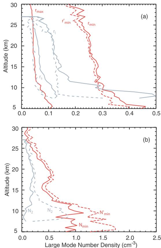
**Fig. 16.** This figure shows the profiles of the Method 1 dependent parameters  $r_{\min}$ ,  $r_{\max}$ , and  $r'_{\min}$  (on frame **a**) and  $N_{\min}$  and  $N'_{\min}$  (**b**) in red. In addition, it shows Method 2 for 3 channels plus a pseudo-infrared channel channels and a free parameters  $r_{I\max}$ ,  $r_{I\min}$ ,  $r_{s\max}$ , and  $r_{s\min}$  (**a**) and  $N_2$  for the maximum SAD (solid) and for the minimum SAD (dashed) in grey (**b**).
