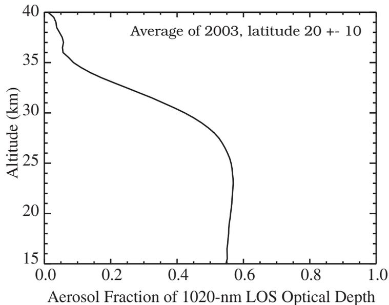
**Fig. 5.** Fraction of the measured slant path optical depth in the 1020-nm channel that is attributed to aerosol. All events between 10° N and 30° N in 2003 are included in the average shown here. Under the conditions of interest the H<sub>2</sub>SO<sub>4</sub>-H<sub>2</sub>O aerosol is expected to fully evaporate at temperatures above ~238 K, corresponding to altitudes between 35 km and 40 km.
