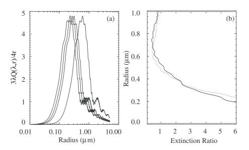
**Fig. 10.** (a) Extinction kernels for SAGE II aerosol extinction channels at 385 (left-most), 452, 525, and 1020 nm (right-most) for spherical water/sulfuric acid drops at stratospheric temperatures. (b) Particle radius as a function of the 525-nm channel to the 1020-nm extinction kernel ratio (or extinction coefficient ratio for a monodispersed aerosol).
