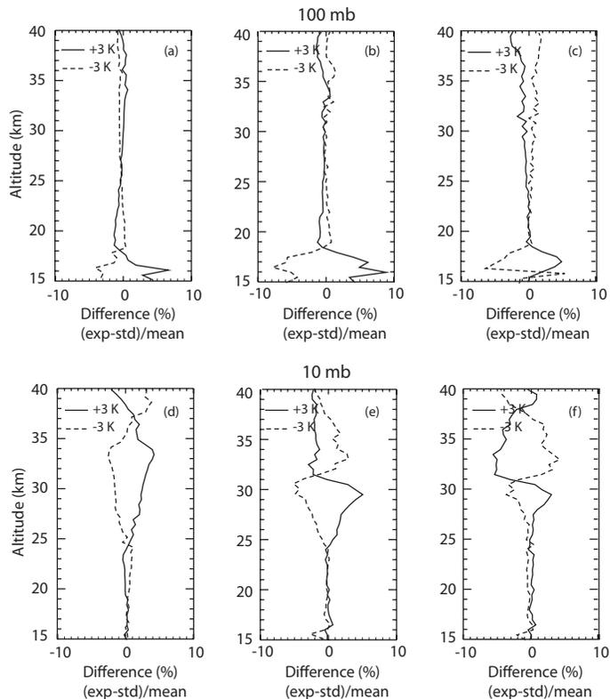
**Fig. 8.** Panels (a), (b), and (c) show the result of perturbing the input temperature value at 100 mb by 3 K (solid lines) and –3 K (dashed). Percent differences for the 1020-nm extinction (a), 525-nm extinction (b) and 525-nm/1020-nm ratio (c) are (experimental - standard)/mean with the meanings as in Fig. 6. Same suite of measurements and cloud clearing is also the same as in Fig. 6. Panels (d), (e), and (f): same at the 10 mb level.
