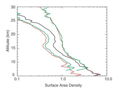
**Fig. 12.** This figure shows a comparison of the operational SAGE II SAD (black) and the SAD computed using Method 1 and 525-nm (red) and 452-nm (green) as the low wavelength aerosol extinction coefficient channel.
