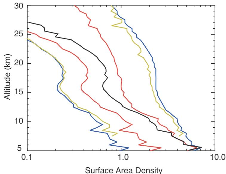
**Fig. 13.** This figure shows the comparison of operational SAGE II SAD (black) with the Method 1 minimum and maximum SAD using 525-nm aerosol extinction coefficient (red) and the minimum and maximum Method 2 SAD using 2 channels at 525 and 1020 nm channels (blue) and 3 channels at 452, 525, and 1020 nm (gold).
