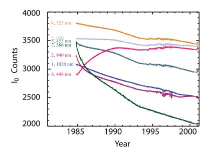
**Fig. 3.** SAGE II exoatmospheric counts for channels 1 through 7 through the lifetime of the instrument. The channels have central wavelengths of 1020, 940, 600, 525, 453, 448, and 386 nm, respectively. The lines are labeled with channel number followed by central wavelength.
