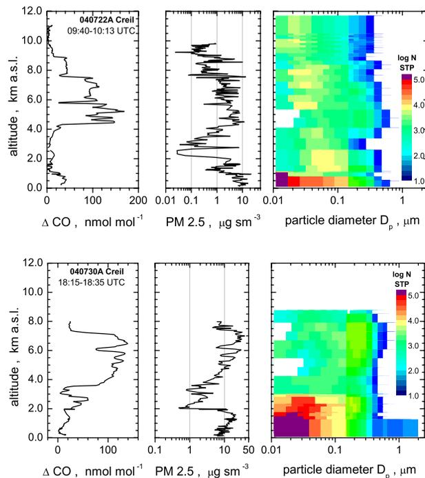
**Fig. 4.** Profiles of excess CO (left), particulate matter mass concentration for standard conditions PM 2.5 (mid), and particle size distribution for standard conditions (right) for Creil on 22 July (ascent) and on 30 July (descent).
