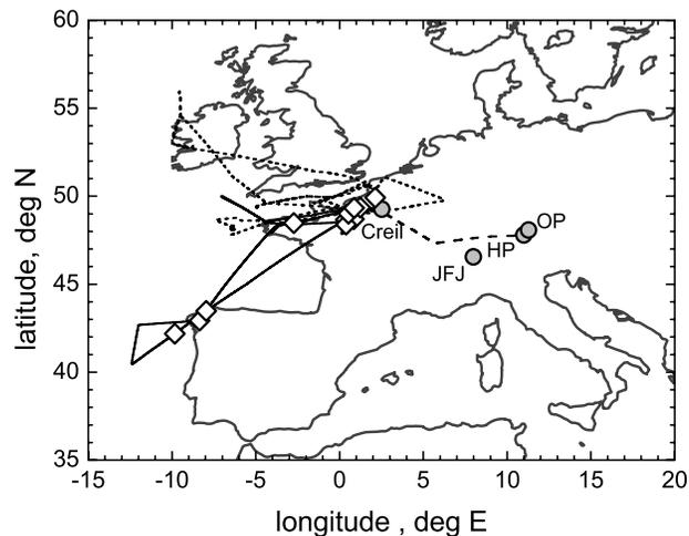
**Fig. 1.** Map of ITOP flights and measurement sites: Oberpfaffenhofen (home base DLR Falcon), OP; Creil (operation base ITOP); Hohenpeissenberg, HP; Jungfrauoch JFJ; open diamonds represent forest fire smoke plume encounters. Performed flights are grouped according to 19 July (dashed), 22–23 July (solid), 25 July, and 26, 30, and 31 July (short dashed).
