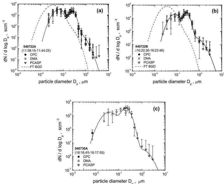
**Fig. 9.** Composite size distributions in forest fire smoke plumes determined from data of Condensation Particle Counters (CPC), a Differential Mobility Anylaser (DMA), and a Passive Cavity Aerosol Spectrometer Probe (PCASP); mission ID and UTC) are given in each plot. Solid lines represent multi-modal log-normal size distributions fitted to the measured data, while the dashed line represents a respective size distribution in the clean UT for the data from 22 July.
