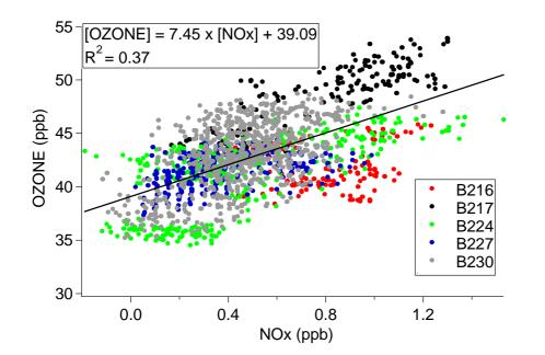
**Fig. 7.** Scatter plot of TECO  $NO_x$  vs. ozone for low level runs from flights in which data is used in Table 1.
