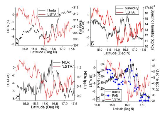
**Fig. 3.** Showing the variation of LSTA and **(A)** potential temperature, **(B)** specific humidity, **(C)** TECO  $NO_x$ , and **(D)** ozone and PAN as a function of latitude during a low level transect over wet features (as described in the text) for flight B224.
