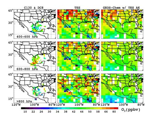
**Fig. 5.** Mean  $O_3$  mixing ratios at 400–600 hPa, 600–800 hPa, and below 800 hPa during MILAGRO/INTEX-B (Phase I). The aircraft measurements are averaged onto 1°×1° grids (left panel). TES data are sampled on the days with aircraft flights and averaged onto 2°×2.5° grids (middle panel). GEOS-Chem results are sampled along the TES orbital tracks with TES averaging kernels applied (right panel).
