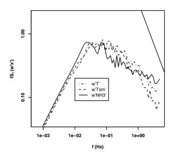
**Fig. 7.** Power spectra of covariance in vertical wind speed with sonic temperature, w'T', smoothed sonic temperature, w'T'<sub>sm</sub>, and fluctuations in NH $_3$  mixing ratio, w'NH $_3$ '. The straight line in upper right shows -4/3 slope expected for fluctuation spectra in an inertial sublayer.
