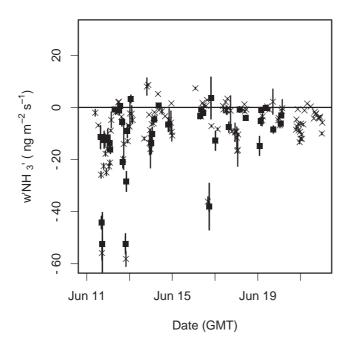
**Fig. 8.** Eddy covariance measurement of NH<sub>3</sub> flux for all time points (crosses) and for those passing quality control criteria for use in calculating deposition velocities (filled squares).
