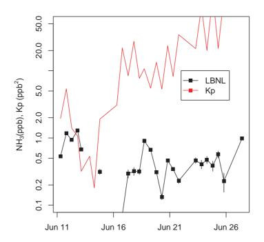
**Fig. 6.** Comparison of  $NH_3$  mixing ratio (black) and aerosol-gas equilibrium partitioning coefficient, Kp (red), indicating minimum product of gas phase  $NH_3$  and  $HNO_3$  mixing ratios necessary for  $NH_4NO_3$  aerosol to be found in equilibrium with gas phase constituents.
