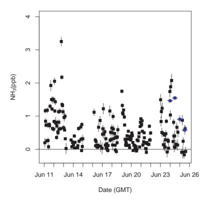
**Fig. 4.** Hourly NH<sub>3</sub> mixing ratios measured at Blodgett Forest in June, 2006. NH<sub>3</sub> data from the laser-spectrometer (black symbols) are averaged into 12 h bins for comparison with integrating filter samples (blue symbols) collected with a sampling system provided by the Desert Research Institute.
