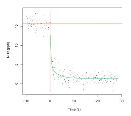
**Fig. 3.** Time series of NH<sub>3</sub> mixing ratio showing transient decay following removal of NH<sub>3</sub> span gas from zero air flow to instrument inlet.
