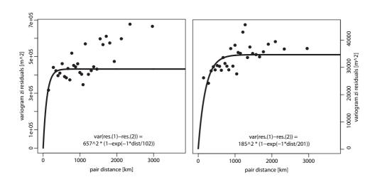
**Fig. 3.** Variogram of mixed layer height residuals  $z_i(ECMWF)$ - $z_i(RS)$  for day (left) and night (right). The lines show a fit with an exponential variogram, for which distances larger then 1300 km where excluded.
