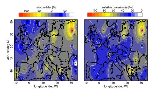
**Fig. 2.** Left: temporally averaged daytime residuals between ECMWF based and radio sounding based mixed layer heights, normalized by the radio sounding based estimate. Right: standard deviation of daytime residuals, normalized by the radio sounding based estimate. Symbols are the same as in Fig. 1.
