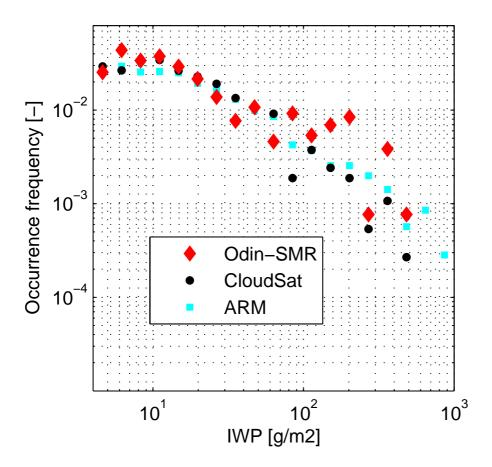
**Fig. 10.** Comparison of pIWP distributions from an area around the tropical ARM stations. Satellite data are taken from a rectangular area, limited of latitudes –9° and 11° and longitudes 142° and 172°. Selection of SMR and ARM data are further restricted to the time period 15 September–15 December (all available years included).
