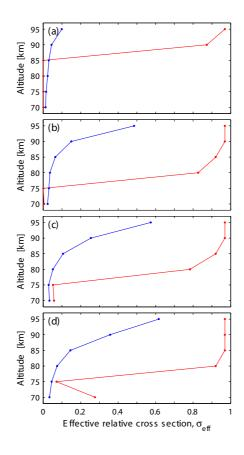
**Fig. 6.** Comparison between the effective relative cross section determined with the Continuum motion model (red lines) and the Brownian motion model (blue lines) for **(a)** 1 nm, **(b)** 2 nm, **(c)** 3 nm, and **(d)** 5 nm radius positively charged particles and the unventilated detector design.
