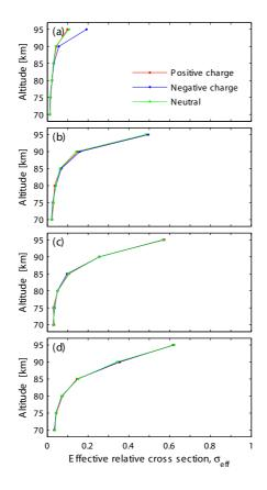
**Fig. 8.** The different effective relative cross sections for positive (red), negative (blue) and neutral (green) particles for **(a)** 1 nm, **(b)** 2 nm, **(c)** 3 nm, and **(d)** 5 nm radius particles and the unventilated detector design.
