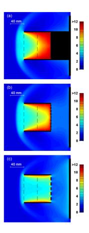
**Fig. 1.** Density field from the DSMC model of the background gas around three detector designs at 75 km altitude normalized to the undisturbed freestream density. The detector designs are **(a)** unventilated, **(b)** ventilated with 10% transmission, and **(c)** ventilated with 50% transmission. The flow is from the left with a speed of 1000 m/s.
