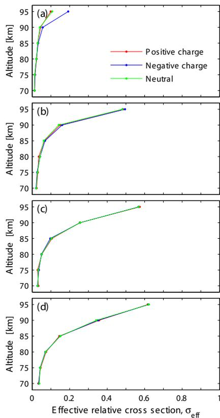
**Fig. 8.** The different effective relative cross sections for positive (red), negative (blue) and neutral (green) particles for **(a)** 1 nm, **(b)** 2 nm, **(c)** 3 nm, and **(d)** 5 nm radius particles and the unventilated detector design.
