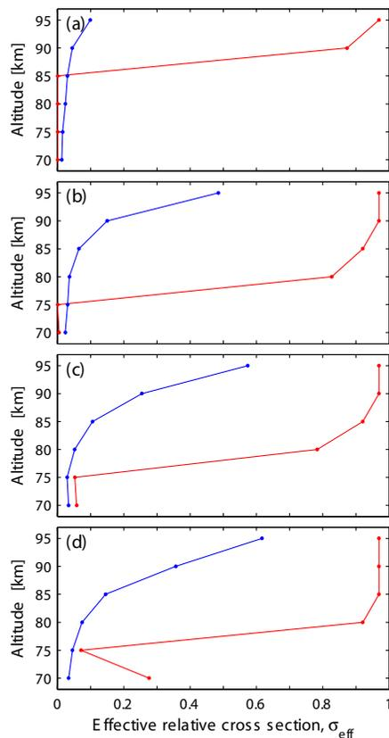
**Fig. 6.** Comparison between the effective relative cross section determined with the Continuum motion model (red lines) and the Brownian motion model (blue lines) for **(a)** 1 nm, **(b)** 2 nm, **(c)** 3 nm, and **(d)** 5 nm radius positively charged particles and the unventilated detector design.
