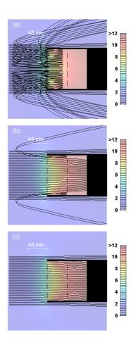
**Fig. 2.** Continuum motion model of **(a)** 0.8, **(b)** 0.9, and **(c)** 1 nm radius positively charged particles approaching the unventilated detector at an altitude of 90 km. The flow is from the left.
