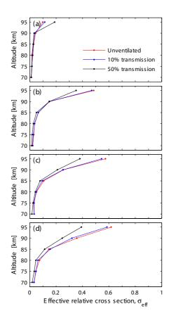
**Fig. 7.** Comparison between the effective relative cross section for the unventilated detector design (red line) and the two ventilated detector designs with 10% (blue line) and 50% (black line) transmission, respectively, for **(a)** 1 nm, **(b)** 2 nm, **(c)** 3 nm, and **(d)** 5 nm radius positively charged particles.
