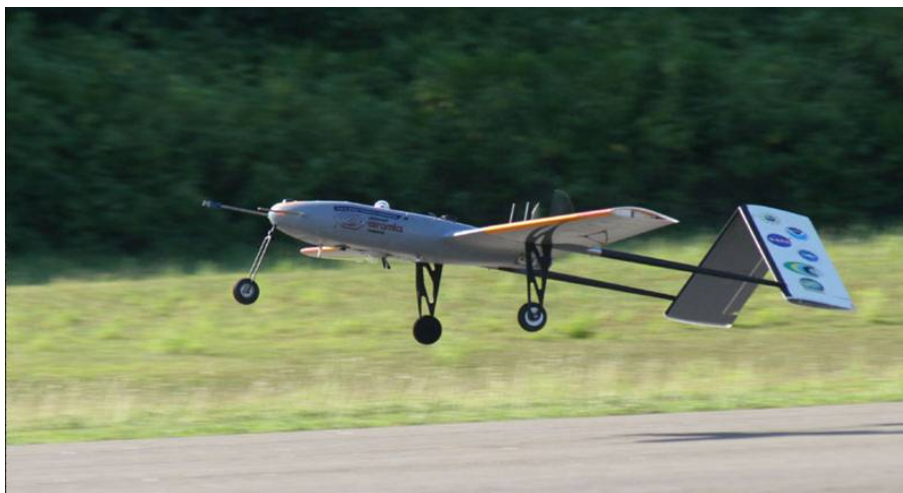
Fig. 2. ACR Manta autonomous unmanned aerial vehicle carrying aerosol-radiation payload landing in the Maldives.
