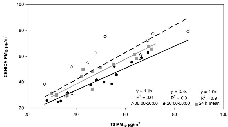
**Fig. 2.** Comparison of 12 and 24 h PM<sub>10</sub> levels simultaneously measured at T0 and CENICA (two urban background sites), Mexico City, during the MILAGRO campaign.
