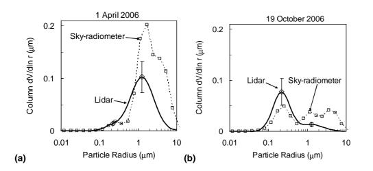
**Fig. 5.** Column particle volume size distributions estimated from the lidar measurements (solid line with diamonds) and those derived from sky-radiometer measurement (dotted line with squares) over Tsukuba on 1 April **(a)** and 19 October **(b)** in 2006. The error bars denote the uncertainties estimated from the lidar signal.
