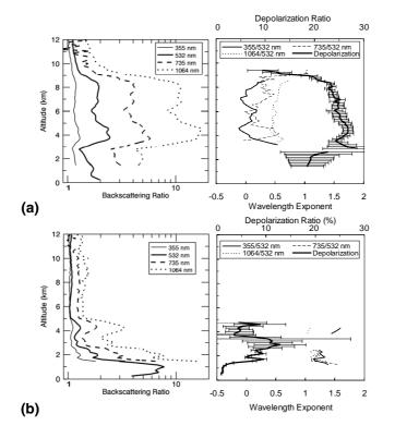
**Fig. 1.** Vertical distribution of the particle optical properties that were obtained with the lidar for the period 00:01–05:03 JST on 1 April 2006 **(a)** and 02:01–06:45 JST on 19 October 2006 **(b)** over Tsukuba. The left panels show the backscattering ratios at wavelengths of 355, 532, 735, and 1064 nm. The right panels show the wavelength exponent of the backscattering coefficients and the particle depolarization ratio at 532 nm.
