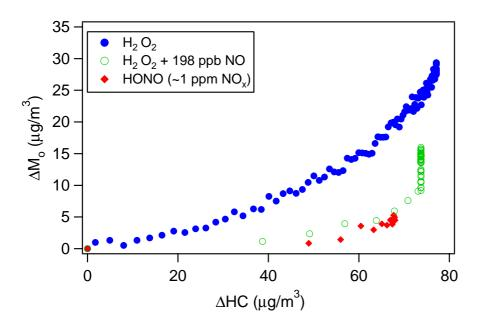
**Fig. 1.** Time-dependent growth curves for  $\alpha$ -pinene photooxidation under different NO<sub>x</sub> conditions (Experiments 1, 3 and 4 in Table 2).
