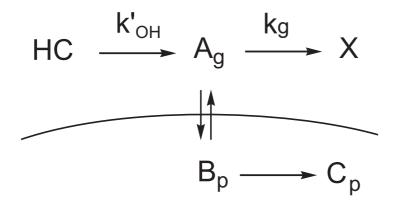
**Fig. 12.** A kinetic scheme depicting the competition between gas-particle partitioning and irreversible loss of the gas-phase semivolatiles. X represents the product of generic loss of semivolatile species  $A_g$  by chemical reaction, and/or loss to chamber walls.  $k'_{OH}$  is the pseudofirst-order rate constant ( $k'_{OH} = k_{OH}[OH]$ ) for photooxidation of the parent hydrocarbon;  $k_g$  is the first-order rate constant of loss of semivolatiles.
