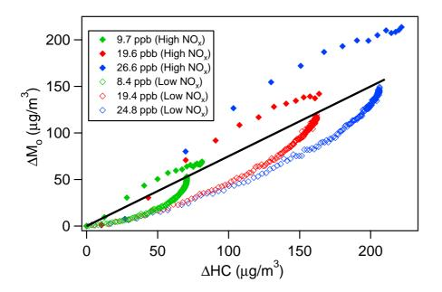
**Fig. 2.** Time-dependent growth curves for longifolene photooxidation under high- and low-NO $_{\rm X}$  conditions (Experiments 2, 3, 4, 10, 11, and 12 in Table 3). The mixing ratios in the legend refer to the amount of longifolene reacted in each experiment. The final SOA yields of each low-NO $_{\rm X}$  experiment lie on a straight line that passes through the origin, indicating that under low-NO $_{\rm X}$  conditions SOA yield is constant, at ~75%.
