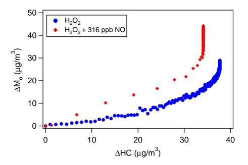
**Fig. 3.** Time-dependent growth curves for longifolene photooxidation with  $H_2O_2$  as the OH precursor. Aerosol growth in the presence of ~300 ppb NO (Experiment 7 in Table 3) significantly exceeds that without NO (Experiment 1 in Table 3).
