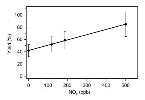
**Fig. 5.** SOA growth as a function of initial  $NO_x$  concentration, at a fixed initial aromadendrene concentration ( $\sim$ 5 ppb). Results shown are given in Table 4.
