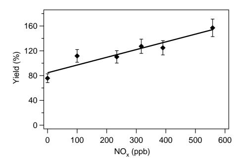
**Fig. 4.** SOA growth as a function of initial  $NO_x$  concentration, for a fixed longifolene concentration ( $\sim$ 4.3 ppb). Results shown are from Table 3.
