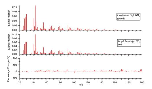
**Fig. 8.** Change in AMS spectrum over the course of longifolene photooxidation under high- $NO_x$  conditions. Top panel: Fractional contribution of each mass fragment to the total organic and nitrate signal during the growth phase of the experiment. Middle panel: fractional contribution of each mass fragment to the total organic and nitrate signal when all hydrocarbon is consumed. Bottom panel: Percentage change of each mass fragment between the growth phase and the end of the experiment.
