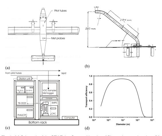
**Fig. 1.** (a) Schematic of the GTK Twinn Ottor and location of Pitot and met-probe tubes; (b) schematic of aerosol Pitot inlet tube; (c) schematic of aerosol instrumentation rack; (d) calculated aerosol losses of air speed of  $0.75 \times 55 \,\mathrm{m \ s^{-1}}$ .
