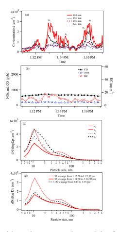
**Fig. 4.** On road ultrafine particle number concentrations and size distributions, 8 October 2004. **(a)** Concentrations of 10.8, 19.1, 29.4 and 52.3 nm particles, **(b)** CO (ppb), NOx (ppb) and BC ( $\mu$ g m<sup>-3</sup>), **(c)** Size distributions at a<sub>1</sub>, a<sub>2</sub>, a<sub>3</sub> and a<sub>4</sub>, **(d)** 30 s and 120 s time-averaging spectra. Note: a<sub>n</sub> are bi-modal size distributions at ~10 nm and ~50 nm and the subscripts reflects different times.
