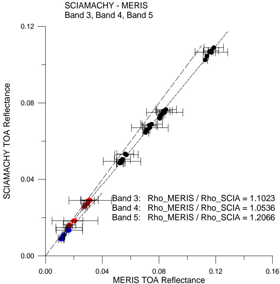
**Fig. 4.** Comparison of TOA reflectance of SCIAMACHY band 3 and band 4 with the MERIS channels 2, 3, 4, 5, 7, 12. The error bars give the standard deviation of the TOA reflectance of the MERIS pixels within one SCIAMACHY pixel.
