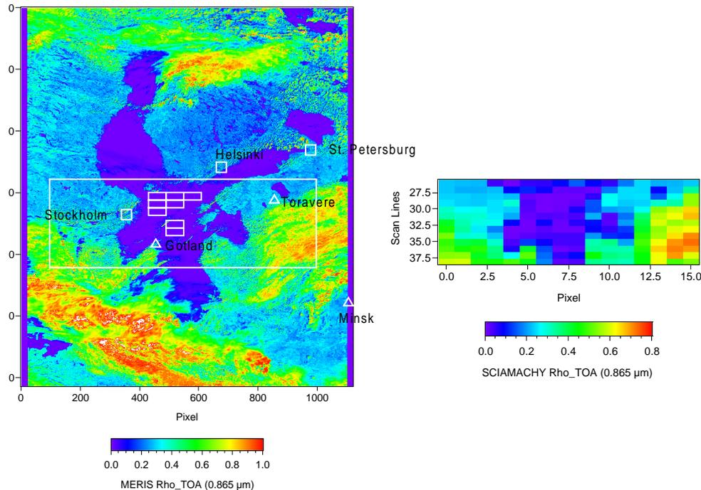
**Fig. 1.** Coinciding MERIS (left) and SCIAMACHY (right) scenes of the 3 August 2002, used for the comparisons. The scenes present the TOA reflectance for the spectral band 0.865 μm. The SCIAMACHY scene and the selected pixels over water of the Baltic Sea without any cloud disturbance are marked by rectangles. The center of the SCIAMACHY scene is located at 58.85° N and 22.03° E. The AERONET sites Gotland, Minsk and Toravere are marked as triangles.
