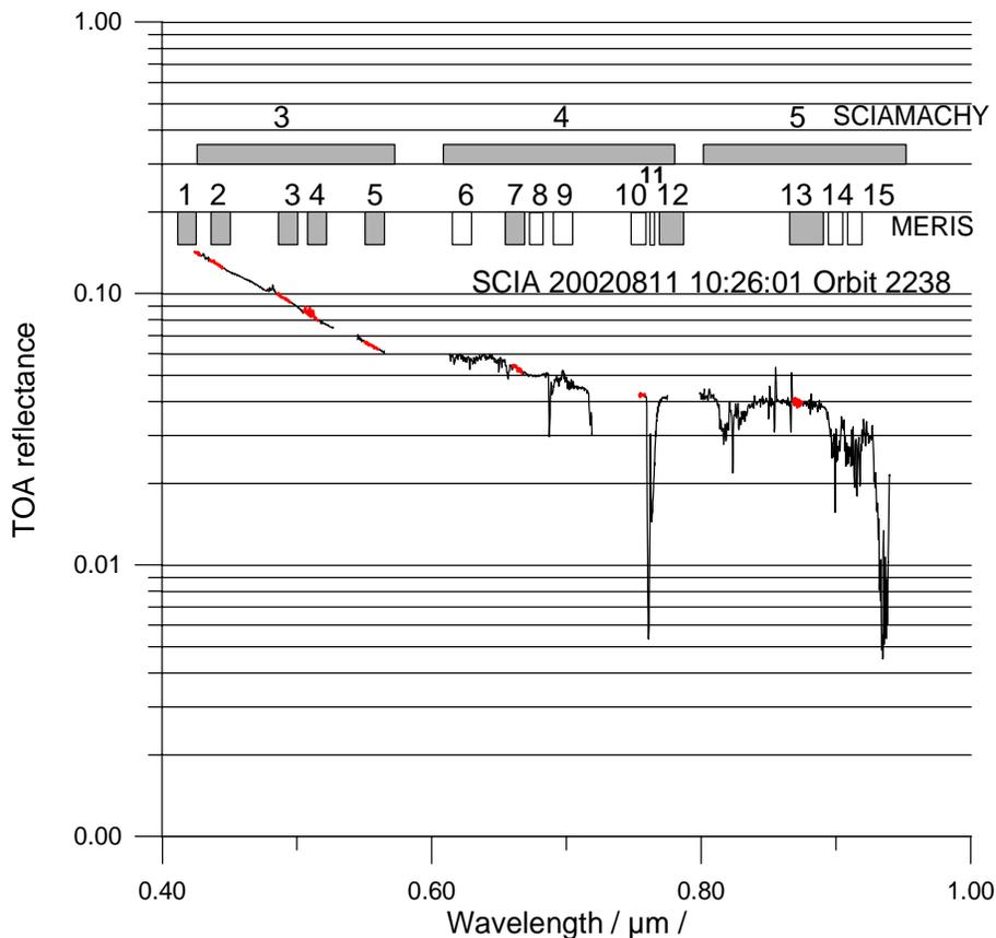
**Fig. 2.** Example of a SCIAMACHY TOA-reflectance spectrum for the bands 3, 4 and 5 and the position of the comparable MERIS channels. The MERIS channels used within the BAER approach are indicate in grey. The available channels of MERIS are indicated in white. The integration regions for the comparisons are shown in red.
