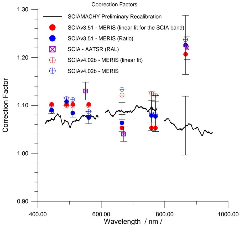
**Fig. 5.** Spectral behavior of the correction factors within the range of SCIAMACHY band 3, 4 and 5. For comparison of correction factors from different approaches the preliminary recalibration of SCIAMACHY and a comparison with AATSR reflectance is combined.
