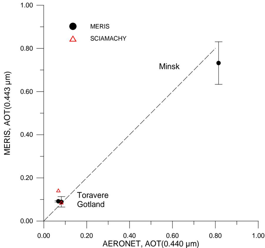
**Fig. 6.** Comparison of AOT for 0.443 μm channel, retrieved from MERIS (black dots) and SCIAMACHY (red triangles) with ground based measurements by the AERONET instruments in Gotland, Toravere and Minsk.
