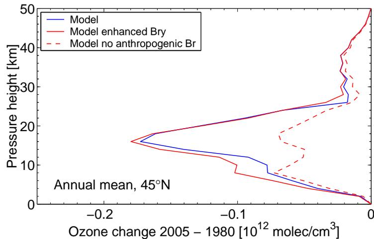
**Fig. 6.** Modelled annual mean ozone change at 45°N between 1980 and 2005 in molecules/cm<sup>3</sup>.
