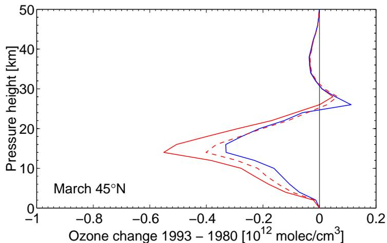
**Fig. 7.** Same as for Fig. 6 but for modelled ozone differences between March 1980 and March 1993. This illustrates that the effect of additional bromine from very short-lived source gases is largest during periods of enhanced stratospheric aerosol loading.
