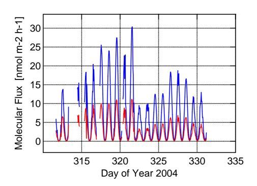
**Fig. 6.** Molecular fluxes of NO<sub>2</sub> (blue line) and HONO (red line) estimated from photolysis of nitrate at Browning Pass during the campaign.
