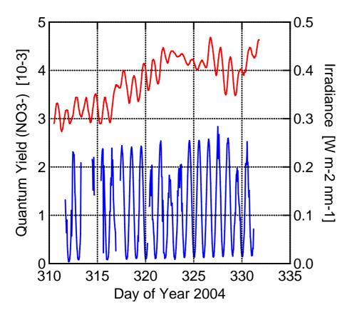
**Fig. 5.** The measured downwelling surface irradiance recorded throughout the campaign at  $350 \, \text{nm}$  (blue, units of W m<sup>-2</sup> nm<sup>-1</sup>, right scale). Also plotted is the calculated quantum yield for nitrate photolysis to yield NO<sub>2</sub> in ice (Reaction R1, units of  $10^{-3}$ , red, left scale). The variation of the quantum yields is due to the temperature of the snowpack recorded at  $12.5 \, \text{cm}$  depth throughout the campaign.
