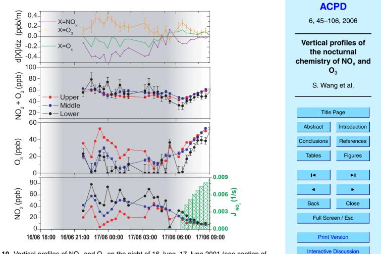
**Fig. 10.** Vertical profiles of  $NO_2$  and  $O_3$  on the night of 16 June–17 June 2001 (see caption of Fig. 9 for a more detailed explanation).
