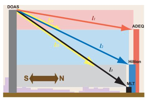
**Fig. 1.** Schematics of the DOAS light paths in Phoenix. The figure also shows the height intervals for which average concentrations were retrieved. The parameters in the figures are explained in detail in Sect. 2.2 and Table 1. The red rectangle refers to the upper box, blue refers to middle box and gray refers to lower box.
