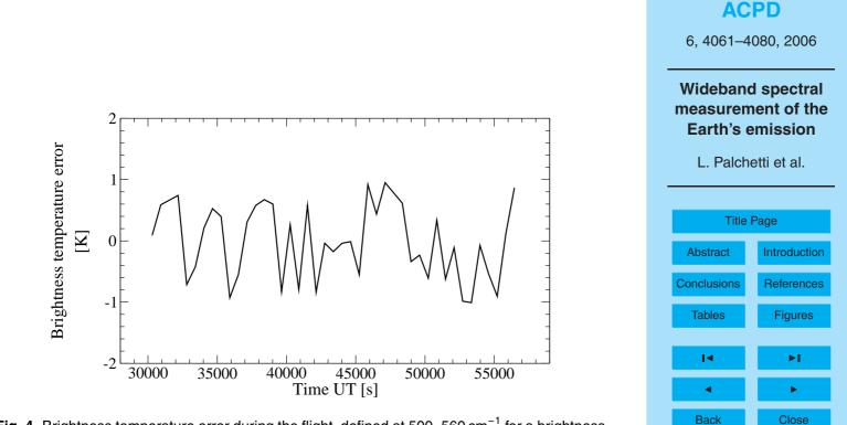
**Fig. 4.** Brightness temperature error during the flight, defined at  $500-560 \text{ cm}^{-1}$  for a brightness temperature of 280 K.
