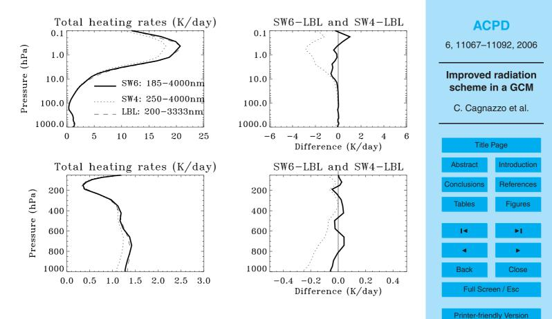
**Fig. 1.** Vertical profiles of total shortwave (SW) heating rates in K/day. Left: SW6, SW4 and LBL are represented with continuous, dotted and dashed lines, respectively. Right: SW6-LBL (continuous line) and SW4-LBL (dotted line) heating rates differences in K/day. Upper panels: from 1000 to 0.01 hPa in logarithmic vertical scale in pressure; lower panels: from 1000 to 10 hPa, linear vertical scale in pressure.
