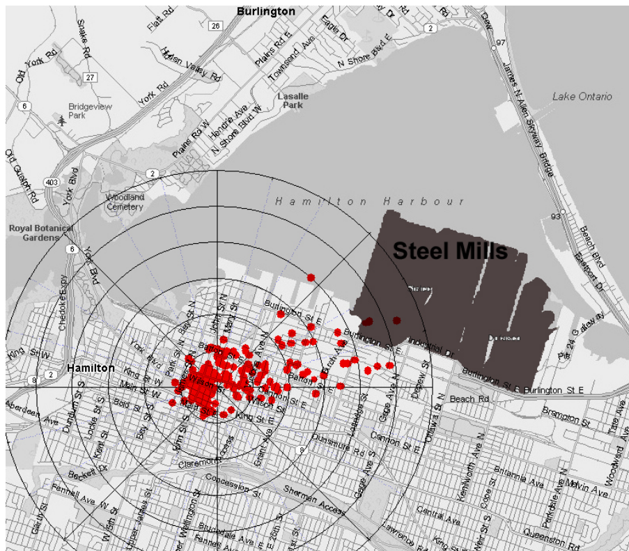
Fig. 7. Polar plot for the local anthropogenic emission factor scores superimposed on a street map of the city Hamilton (map source: http://mappoint.msn.com ). Each radial increment represents the relative magnitude of the absolute factor scores. The measuring site is represented by the center of the polar plot. The dark grey area indicates the two large steel mills in Hamilton.
